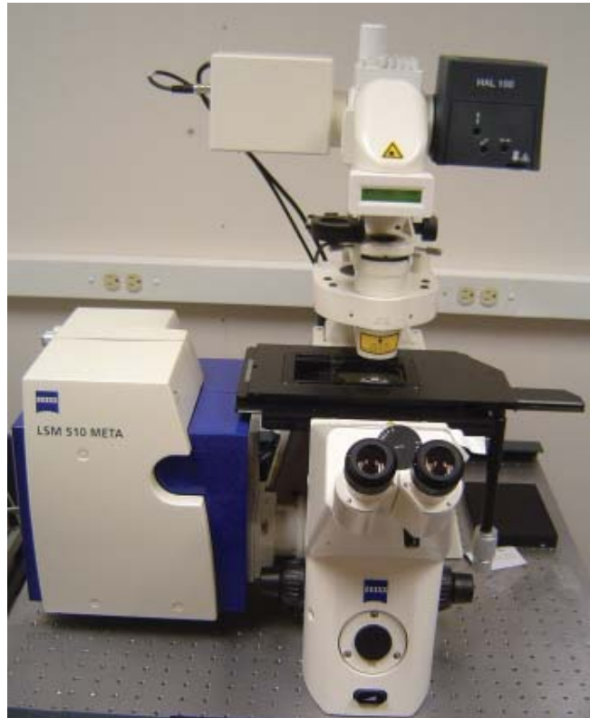
Figure 4.11: Laser scanning confocal microscope for capturing the images (photo taken in WSU's Franceschi Microscopy and Imaging Center).
