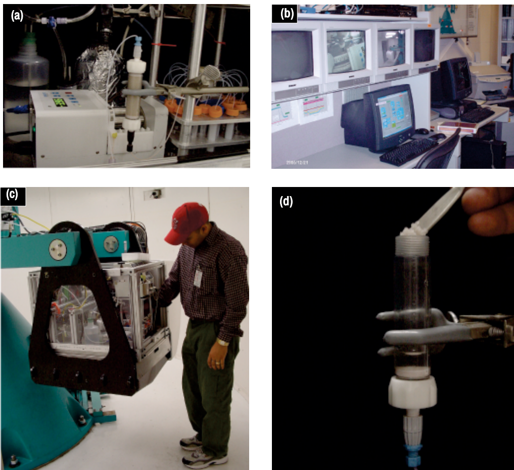
Figure 2.1: The 50 g-ton, 2-m radius geocentrifuge at the Idaho National Laboratory in Idaho Falls, ID. (a) platform, (b) control room, (c) overview, (d) column filling.
