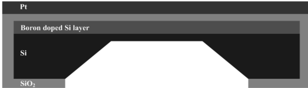
Figure 3-8: A schematic view after sputtering Pt layer.
