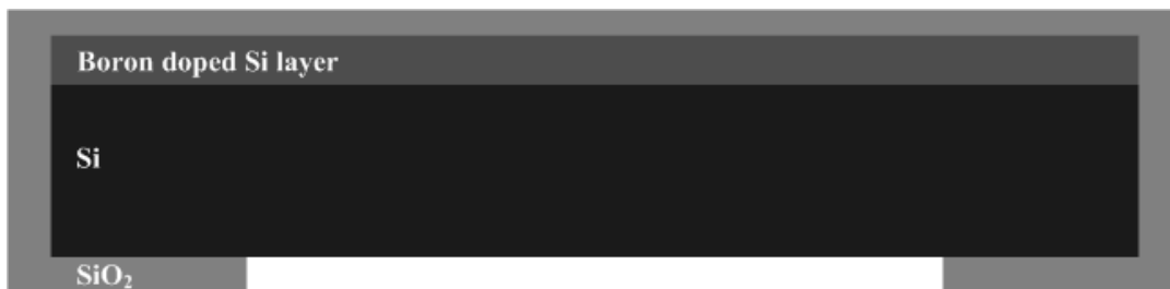
Figure 3-5: Silicon wafer after pattern etch mask for EDP etching.
