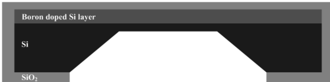
Figure 3-6: Schematic view of a fabricated membrane after EDP etching.
