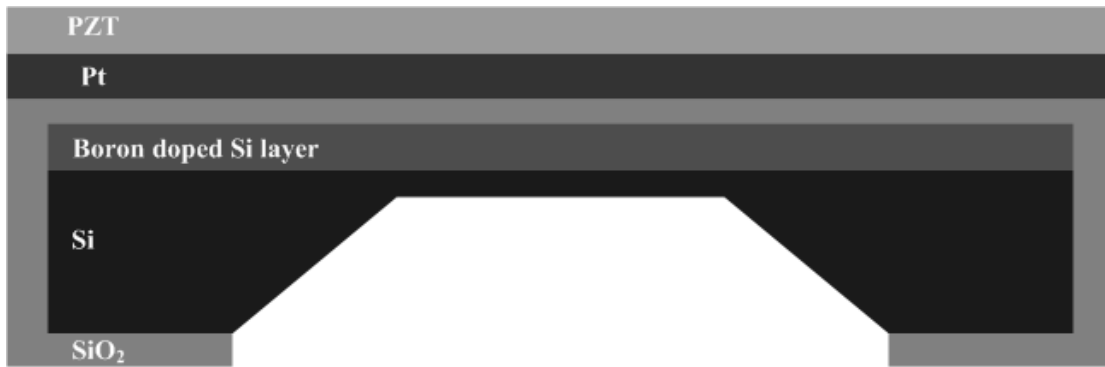
Figure 3-9: A schematic view of a membrane after PZT deposition.
