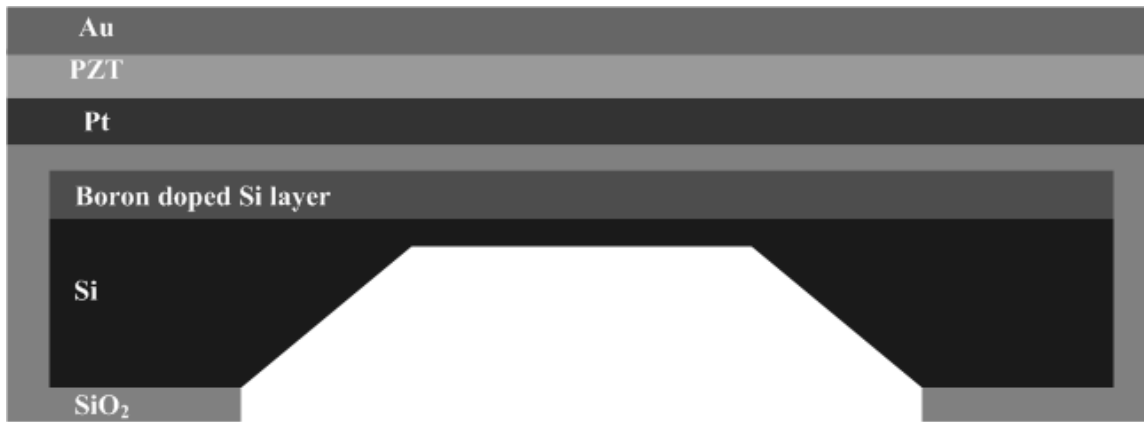
Figure 3-10: A schematic view of a membrane after top electrode sputtering.
