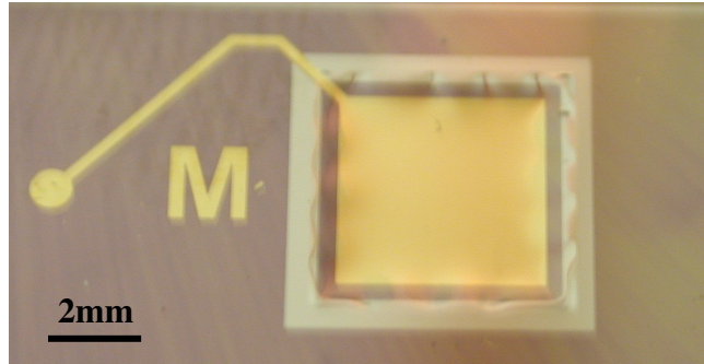
Figure 6.5: Optical image of a low stress 5 mm membrane that has a PZT etch pattern that extends around almost the entire membrane edge.
