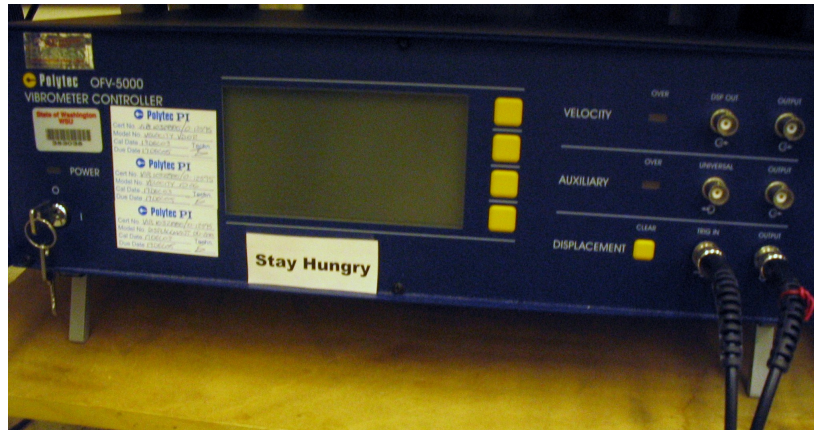
Figure 7: The main controller of the laser vibrometer.
