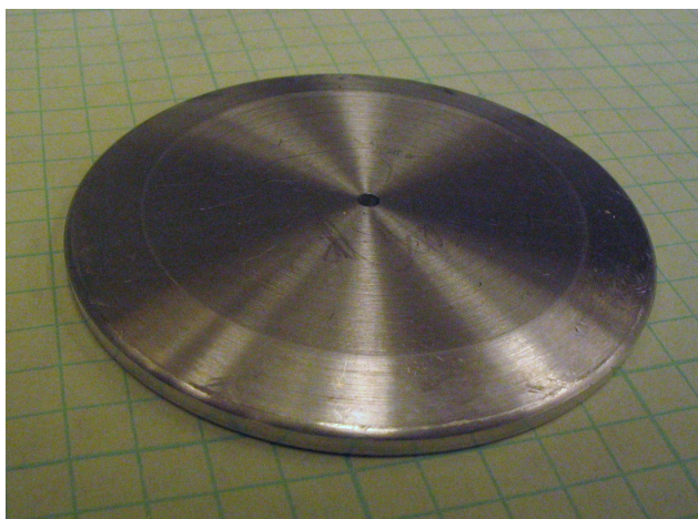
Figure 4: A typical puck that is used for testing a single membrane.
