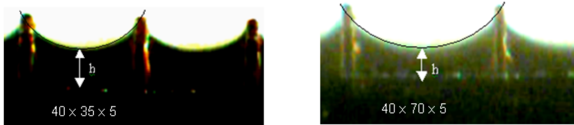
Figure 5.17 Microphotograph of micro-channels with working fluid, FC77
