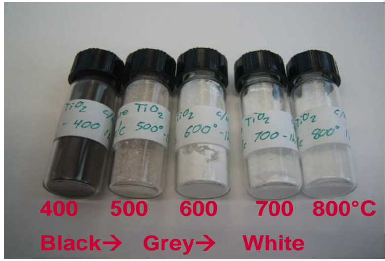
Figure 3.1. Photograph of the calcined TiO 2 nano-powder showing the color varying from black to white.
