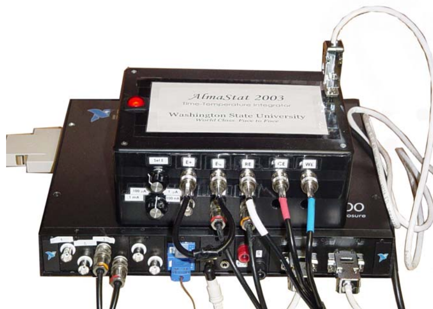
Figure 3. Potentiostat (AlmaStat 2003) data acquisition connector box
