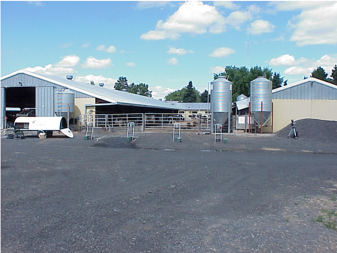
Figure 4.2: North milking stalls with spectrograph and light source in the trailer, retroreflectors on the right, tracer gas syringe samplers on the stands, during tracer experiment.
