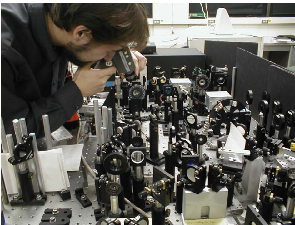
Figure 3.2: The pump-probe apparatus used to investigate the vibrational dynamics associated with excitonic self-trapping.
