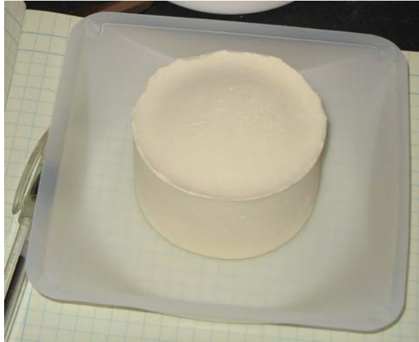
Figure 6.1: Calcined PMN-PT charge after being pressed in isostatic press
