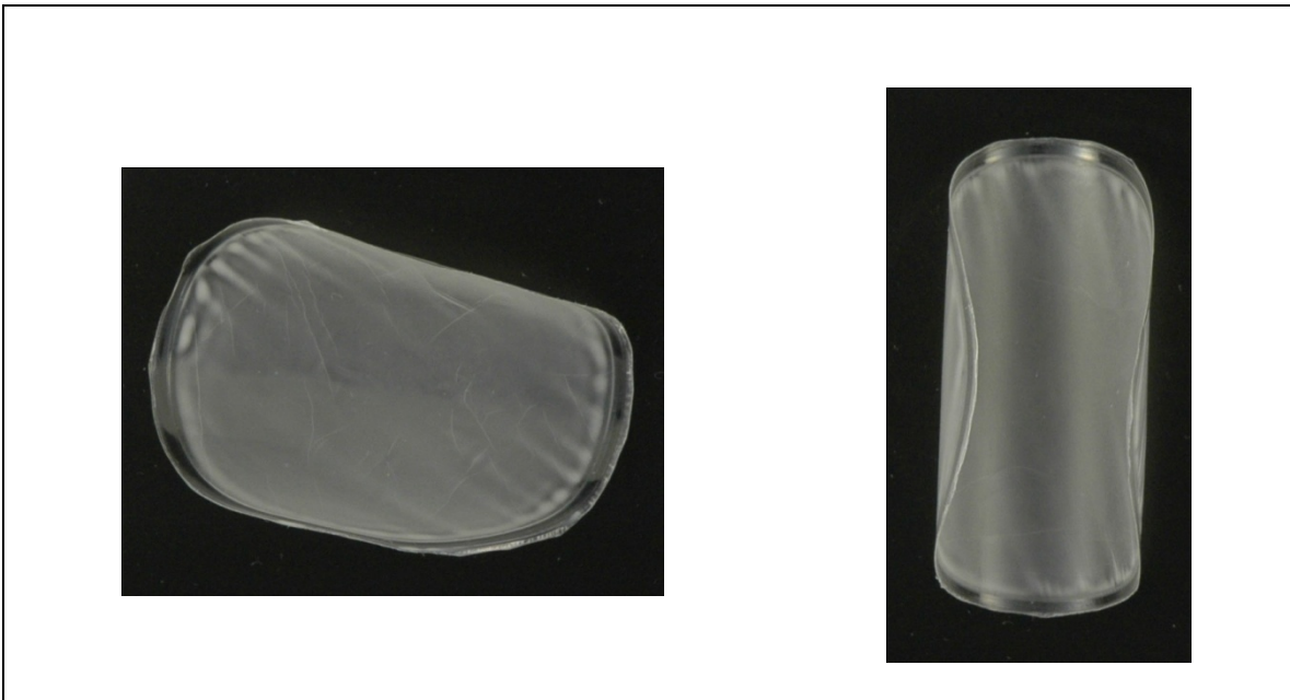
Figure 4.3. Film specimens after retort showing clear region along location of O -rings
