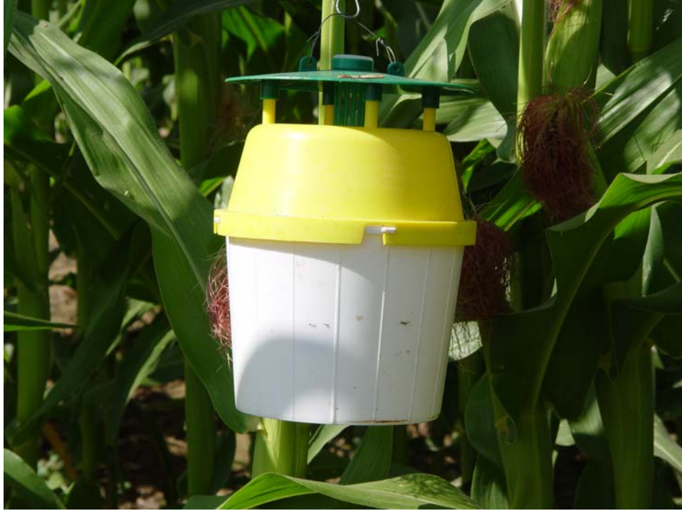
Figure 1: Universal Moth Trap™ used in field experiments with green lid, yellow cone, and white bucket.
