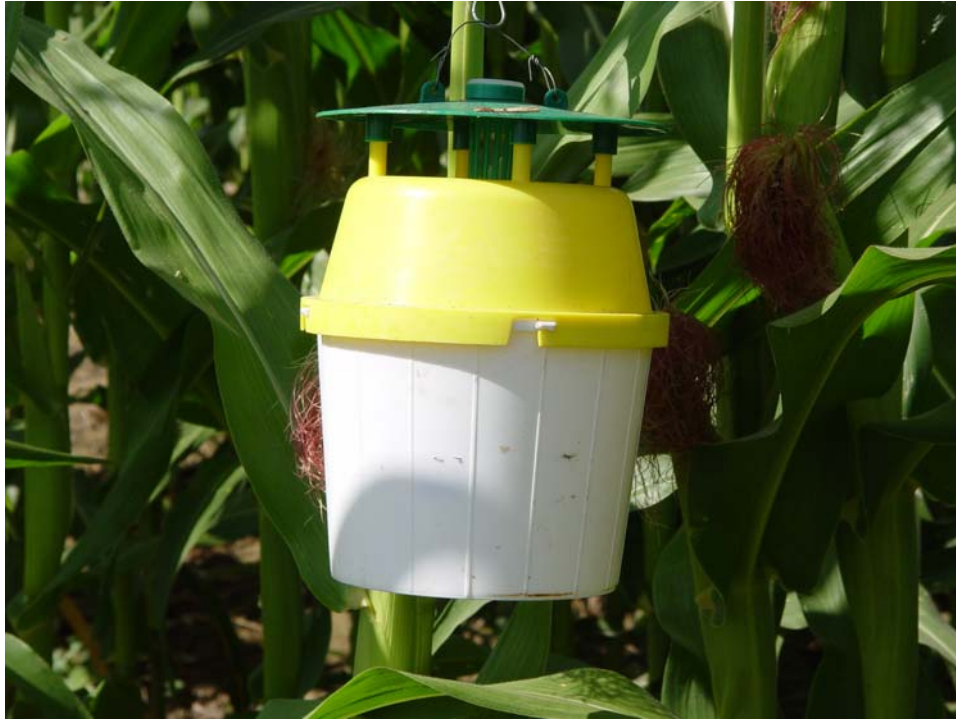
Figure 2: Universal Moth Trap™ used in field experiments with green lid, yellow cone, and white bucket.
