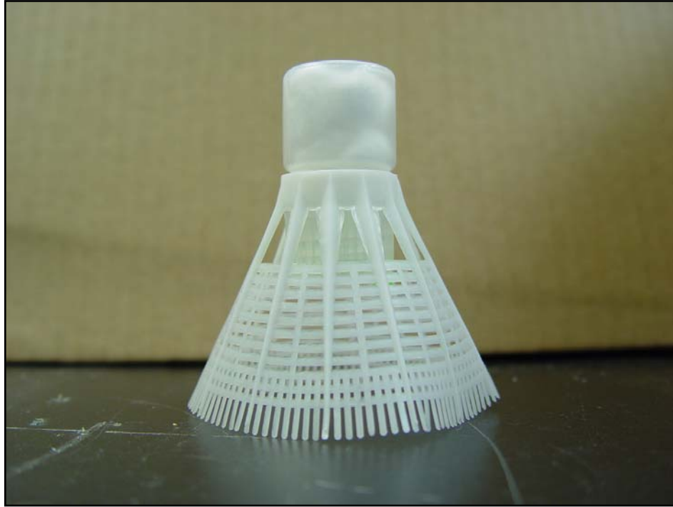
Figure 2: Shuttlecock (badminton birdie) killing stations combined with 8.0 ml Nalgene™ vial.
