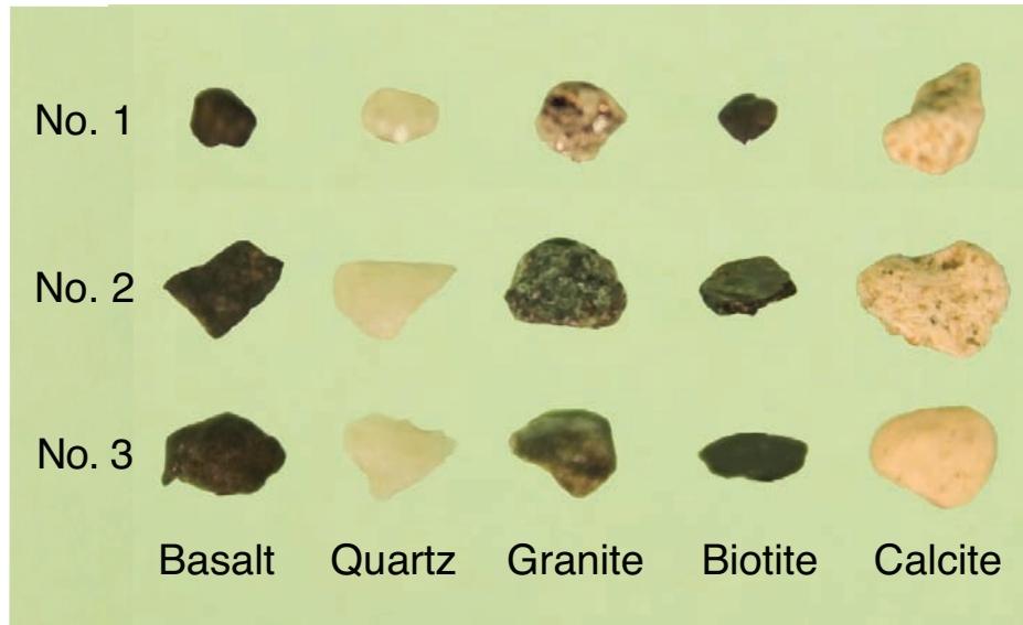
Figure 5.4: Five different natural Hanford sediment particles (basalt, quartz, granite, biotite, and calcite) with irregular shapes.
