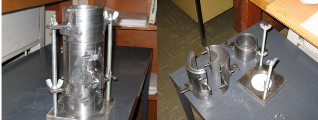
Figure 3.8: Custom built mold for triaxial test.
