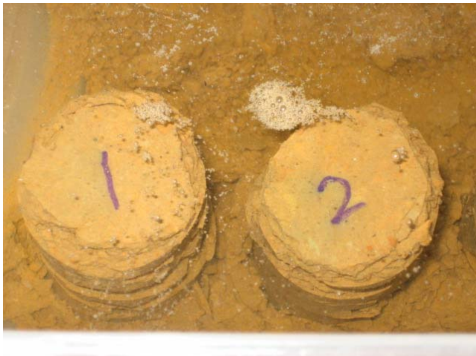
Figure 4.11: Disintegration of specimens after being immersed in water.
