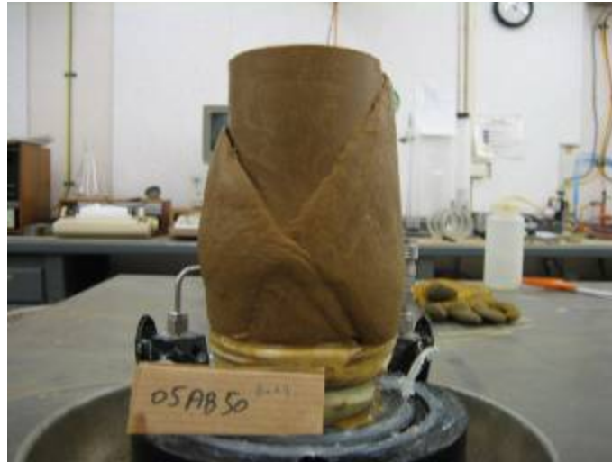
Figure 4.29: Planar type of failure for 5% cement treated Aberdeen soil.
