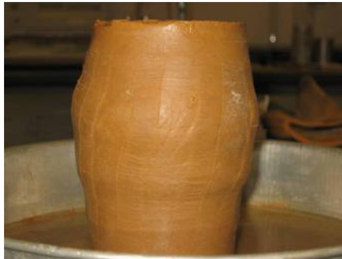
Figure 4.28: Ductile type of failure for non-treated Aberdeen soil.
