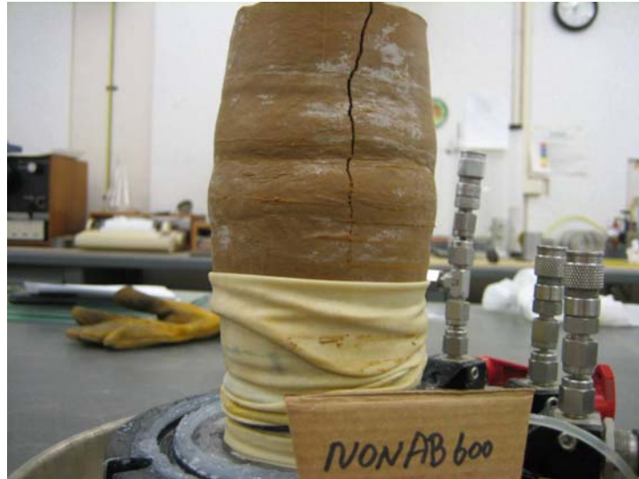
Figure 5.9: Ductile type of failure with vertical crack for non-treated Aberdeen soil.
