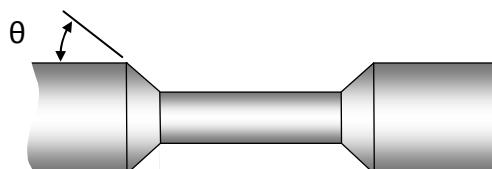
**Figure 45. 1.0 ft. long 1.0 in. diameter rods with multiple transition angles used for detection of simulated corrosion**
