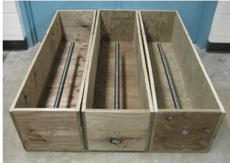
**Figure 59. Boxes constructed for signal attenuation tests in soils**
