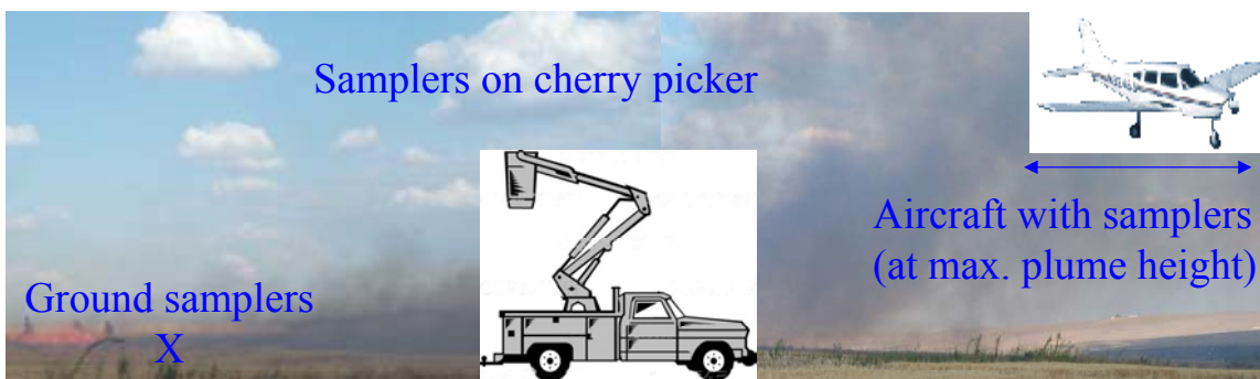
Figure 6.2: Proposed field experiment to study the effects of smoke aging (cliparts from http://www.fotosearch.com ).
