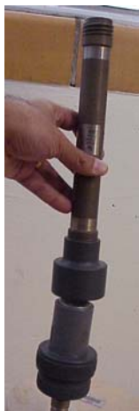
Figure 6.3: O_3 denuder on PM_{2.5} sampler.
