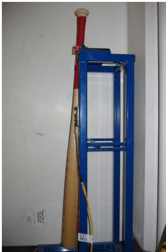
Figure 1.2: Fixture used to measure the moment of inertia of a bat. The pivot clamp is located 6'' from the knob end of the bat.
