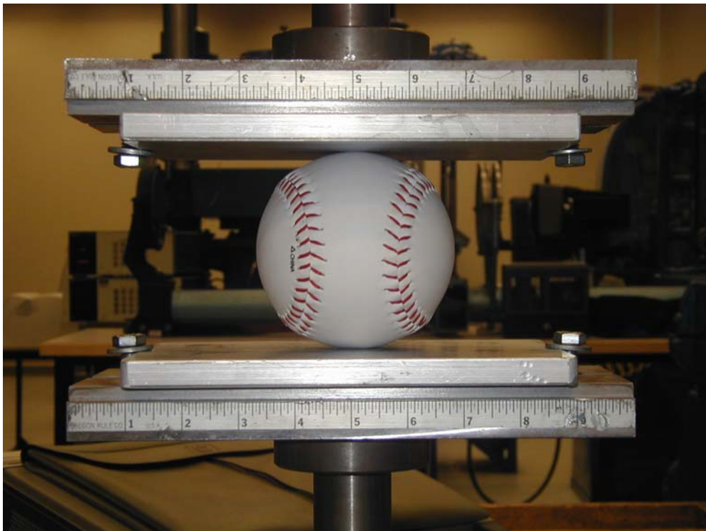
Figure 2.8: Picture of static compression load frame (MTS Systems Corporation, Minneapolis, MN).
