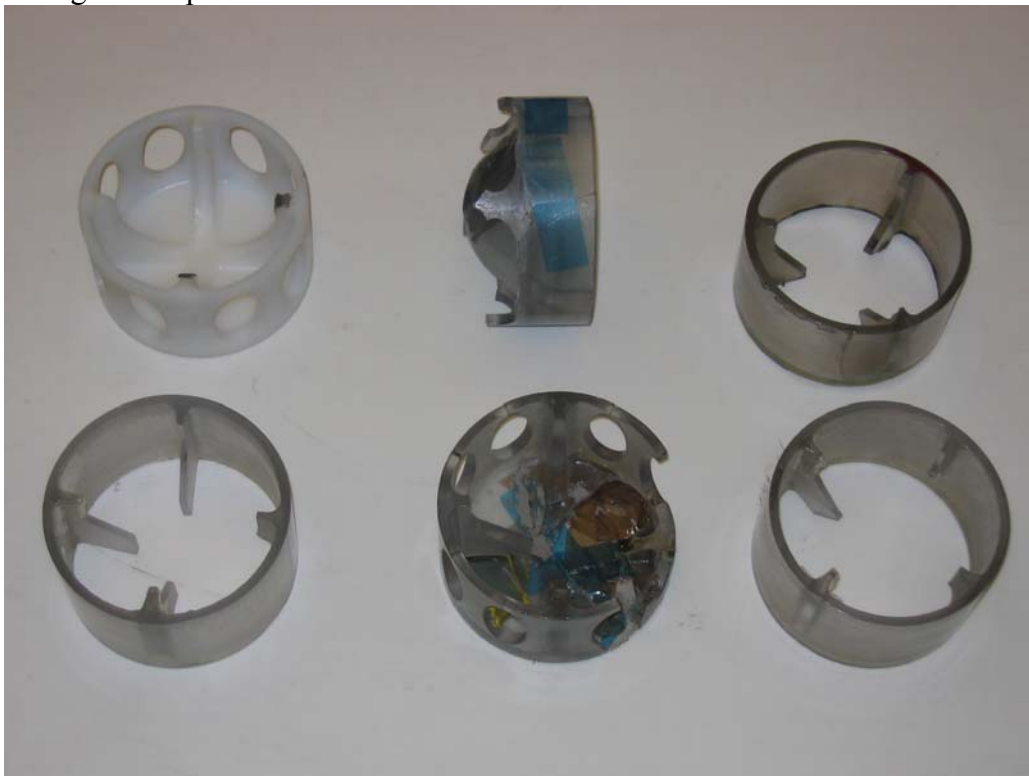
Figure 2.6: Several sabot designs that failed with repeated impacts. The original UHMWPE design is shown in the upper left. The others are made of polycarbonate.
