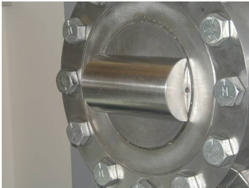
Figure 2.36: Picture of cylindrical impact surface attached to strain gage load cell. Cylindrical impact tests were also performed using piezoelectric load cells.
