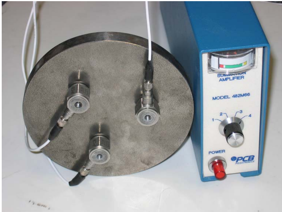
Figure 2.20: Picture of piezoelectric load cell experimental setup. The load cells are mounted in an equilateral triangle with a common side length of two inches.
