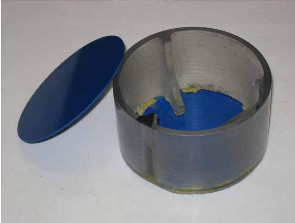
Figure 2.7: Picture of the current sabot design with the fiberglass bottom plate. An example of the 1/16" backing plate is shown also.
