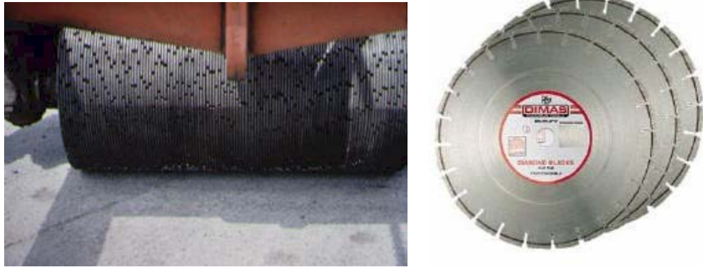
Figure 1.3 Gang Mounted Diamond blades (left). Close up View of Diamond blades (right).
