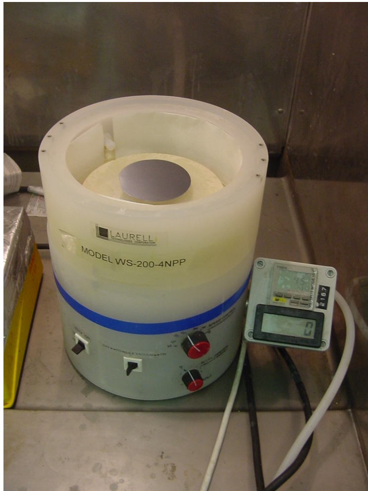
Figure 2.7: A picture of the spin coating machine. The silicon wafer is placed in the center of the machine on a spindle, and held in place with vacuum through the spindle.
