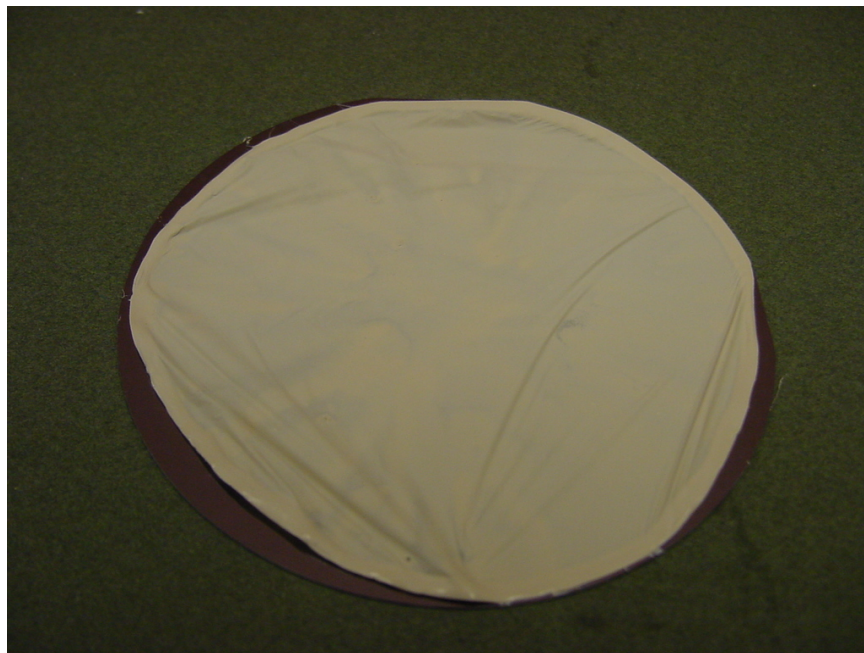
Figure 2.14: The figure above is of a finished composite sample approximately 20 \mu\text{m} thick. Each type of film sample peels away from the silicon wafer after several days of drying.
