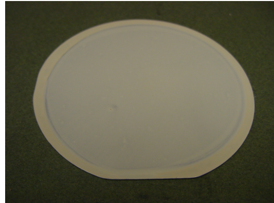
Figure 2.9: A composite film showing the resulting 'ring' of excessive thickness when the sample is spun too fast.
