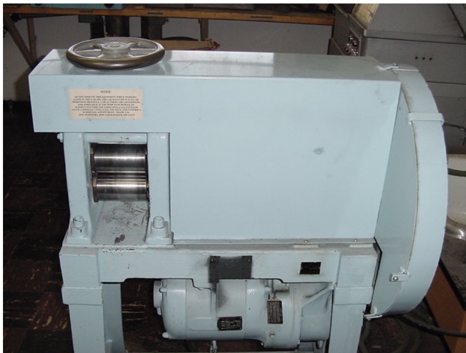
Figure 2.3: A figure of the steel roller used to roll polymer and composite samples.
