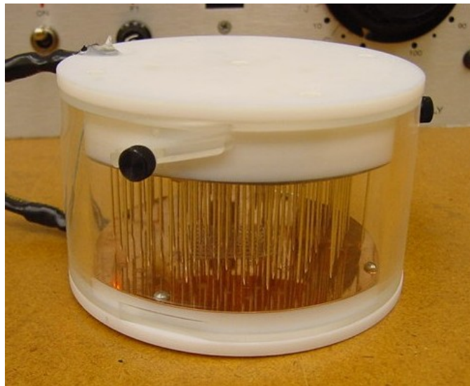
Figure 2.10: The Corona Poling Station. This is connected to a DC power supply to create an electrical field between the steel needles and the bottom copper plate necessary for poling.
