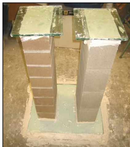
Figure 3.5: Capping with gypsum cement
