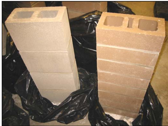
Figure 3.3: Both kinds of piers before being grouted and sealed in the plastic bags
