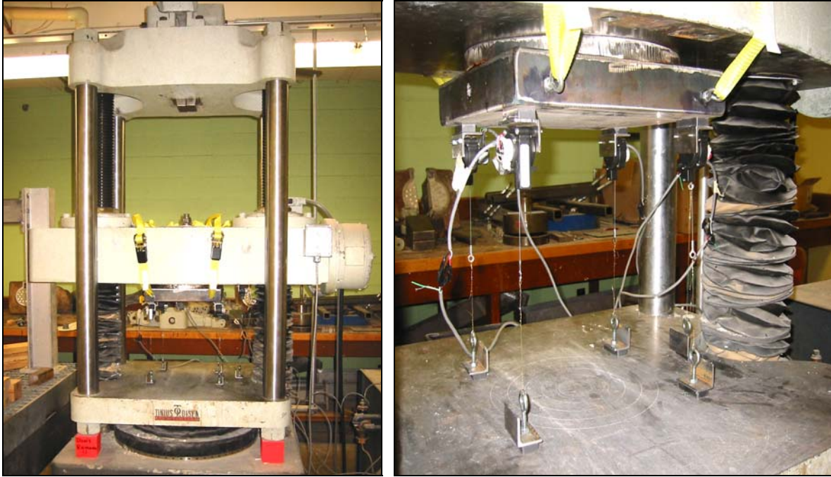
Figure 3.6: 400-kip Tinius Olsen Universal Testing Machine (left) and details of the bearing plate and potentiometers (right)
