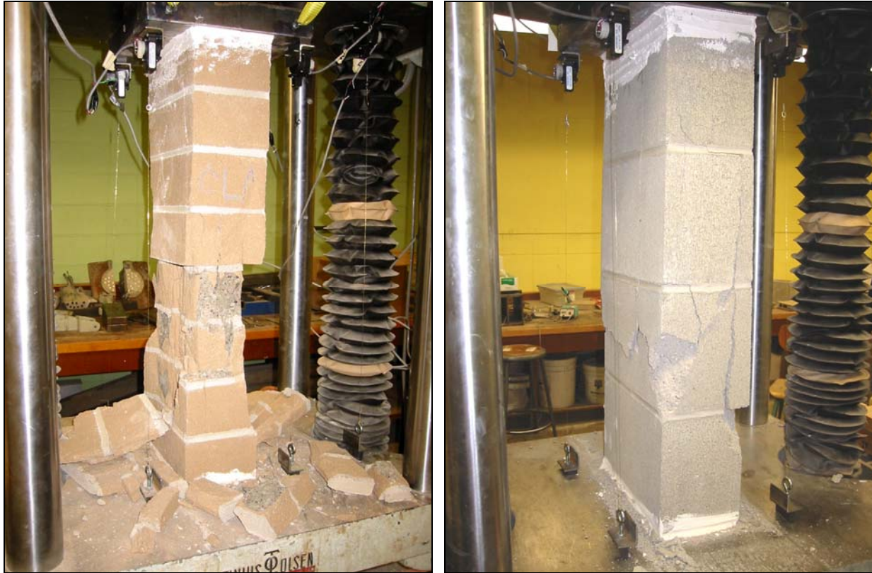
Figure 3.7: Unreinforced clay masonry pier (left) and reinforced concrete masonry pier (right) after testing
