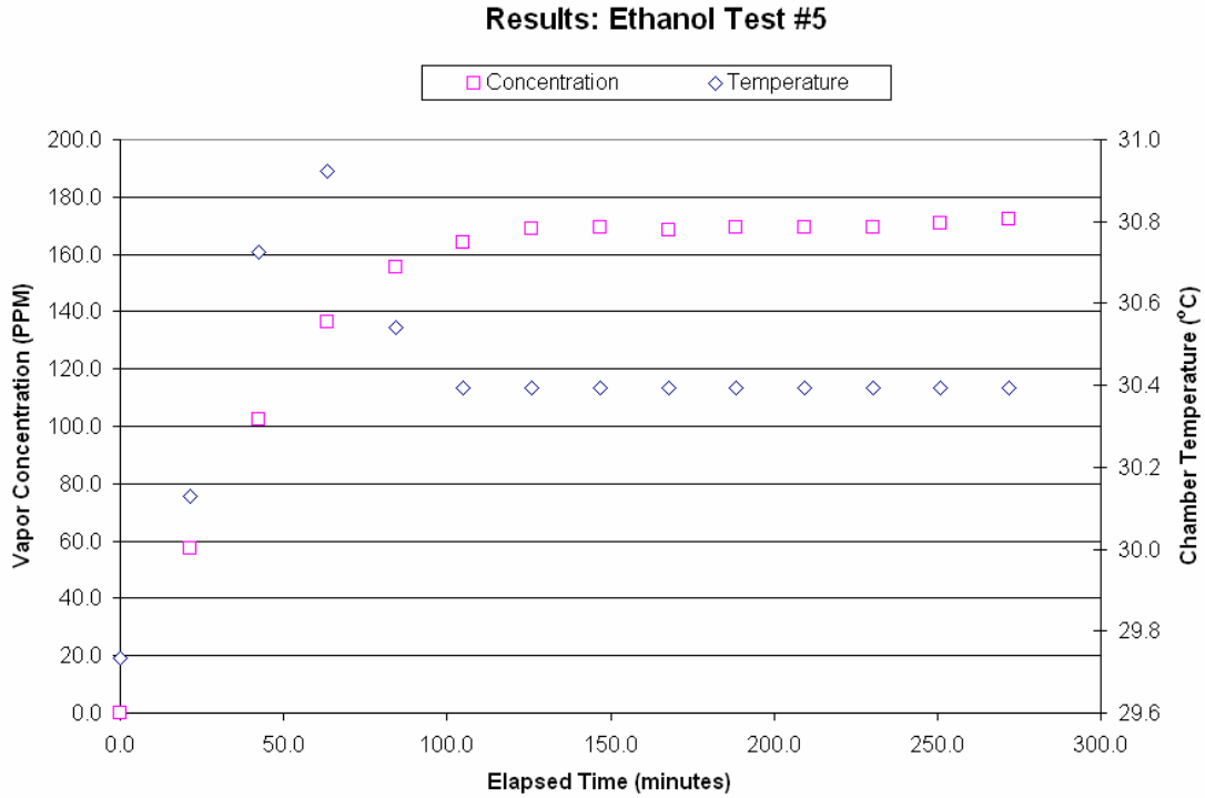
Figure 37: Concentration and Temperature Profile Data of Ethanol Test #5
