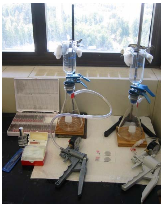
Figure C7: Filtration and enumeration set up for field samples
