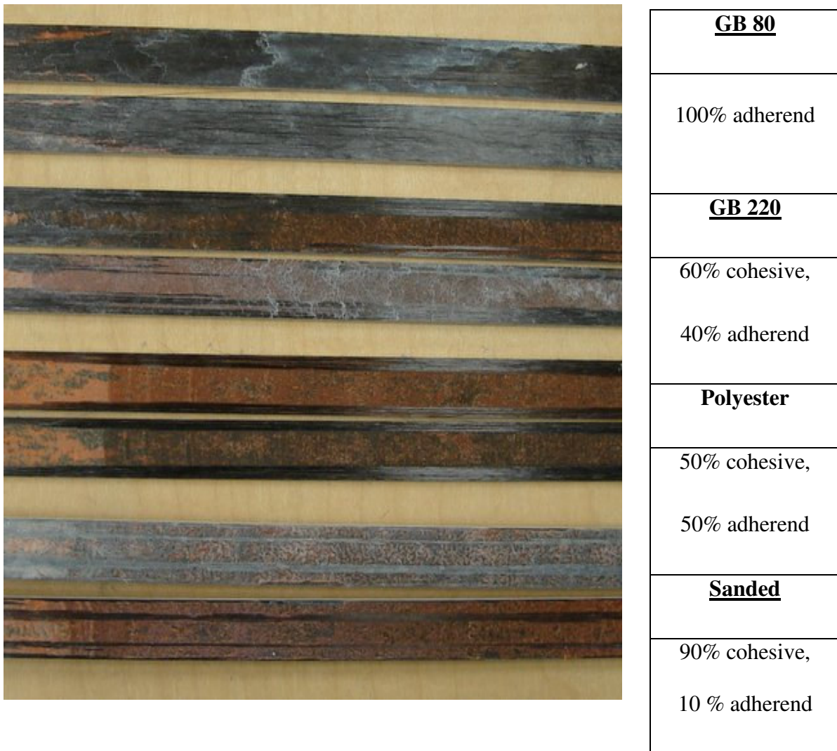
Fig 5.23) Failure modes of DCB specimens resulting from fluctuating load test. Load applied is 9.5 lbs on all specimens.
