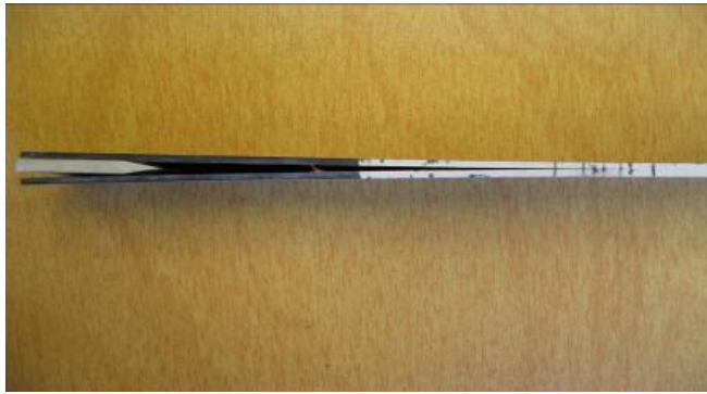
Fig 4.6) Crack measurement of an edge painted WC specimen
