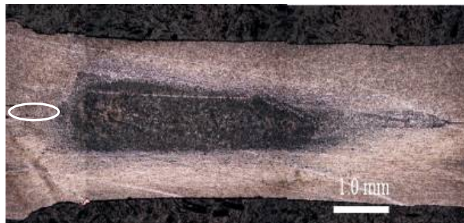
(b) POST-WELD COLD WORKED (4.6 MM IS, 450 MPA IP)
