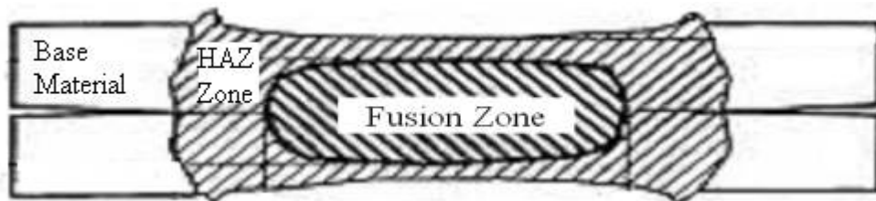
FIGURE 2.3. RSW CROSS-SECTION SCHEMATIC.
