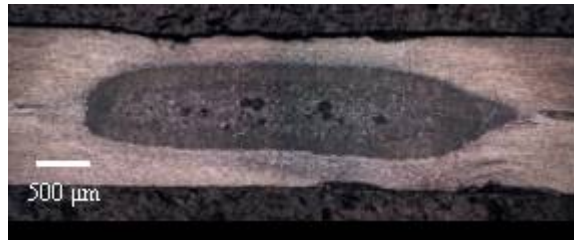
FIGURE 2.5. AL RSW CROSS SECTION.
