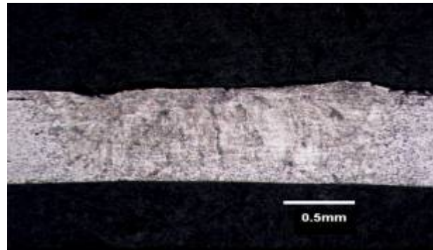
(b) SIDE VIEW OF FAILURE TYPE A (LOWER SHEET ONLY)
