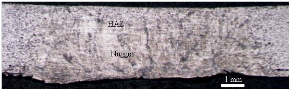
FIGURE 5.3. MICRO-STRUCTURE OF STEEL RSW.
