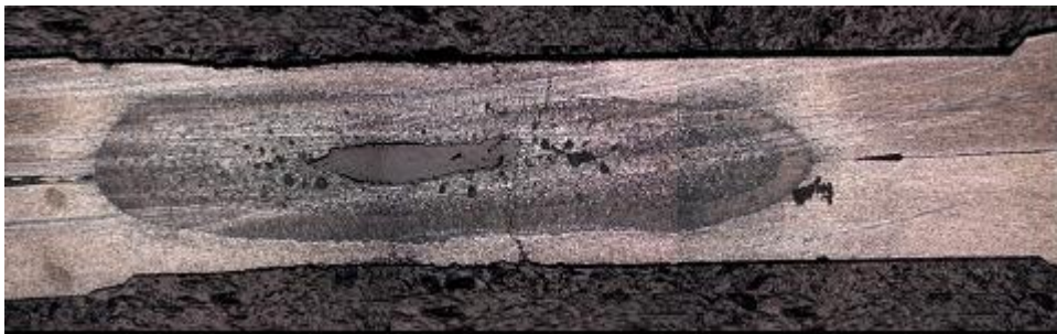
Microstructure of Al 5052 RSW with cold working parameters of IS 7.1 mm and IP 450 MPa
