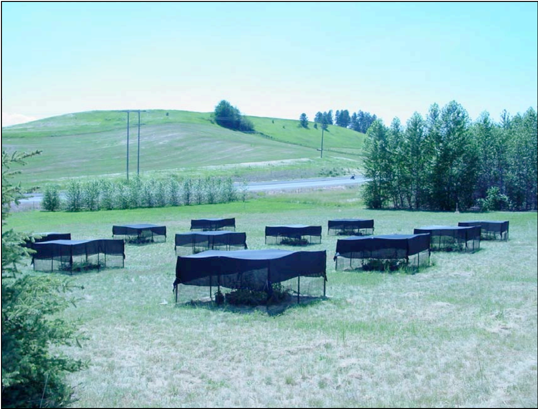
Figure 1. Shade experiments on the Washington State University campus. Shade structures were spaced so as to prevent shading by a nearby structure.
