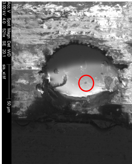
(a) Ga droplet after micro Vickers hardness test
