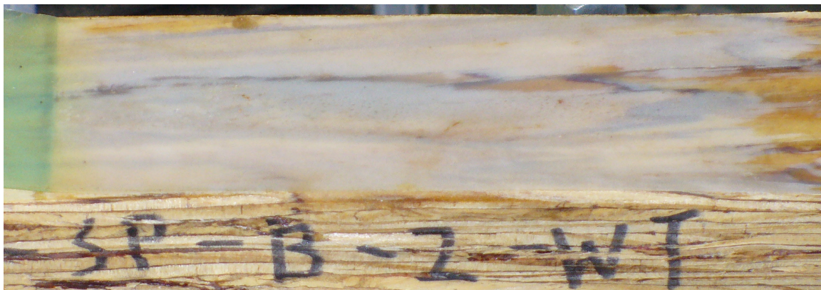
Figure 3-9: Delamination between HDPE barrier layer and wood composite specimens bonded with tie-layer B after aging test.
