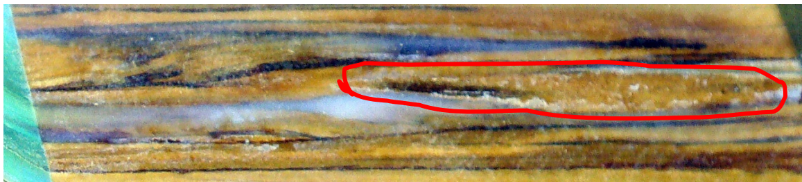
Figure 2-8: Signs of HDPE degradation on 200°C specimen
