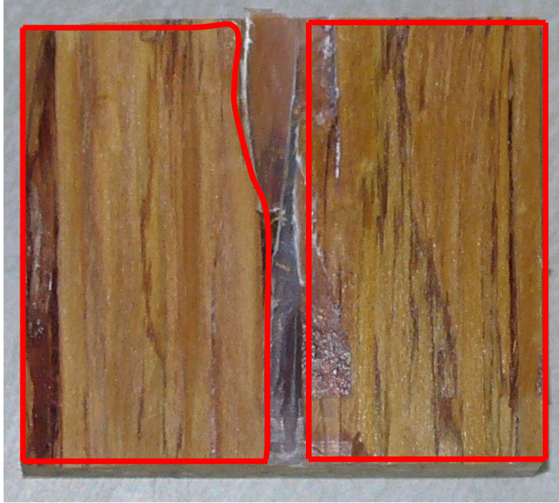
Figure 3-10: Wood failure after block shear test bonded with tie-layer A.
