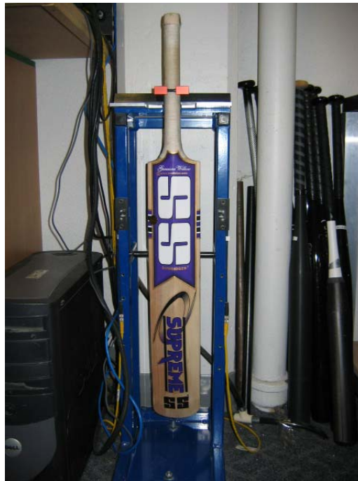
Figure 4.2: Experimental apparatus used to measure the MOI of the cricket bat.
