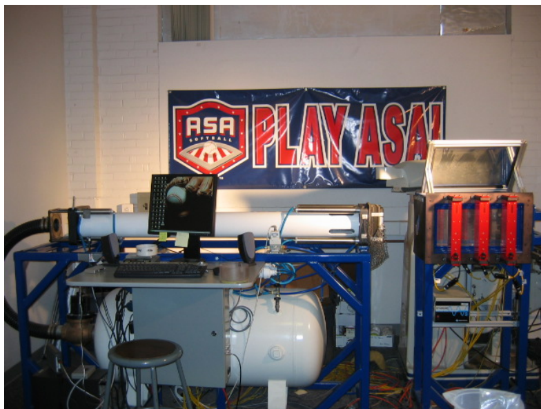
Figure 4.3: Experimental test fixture used to test cricket bats.
