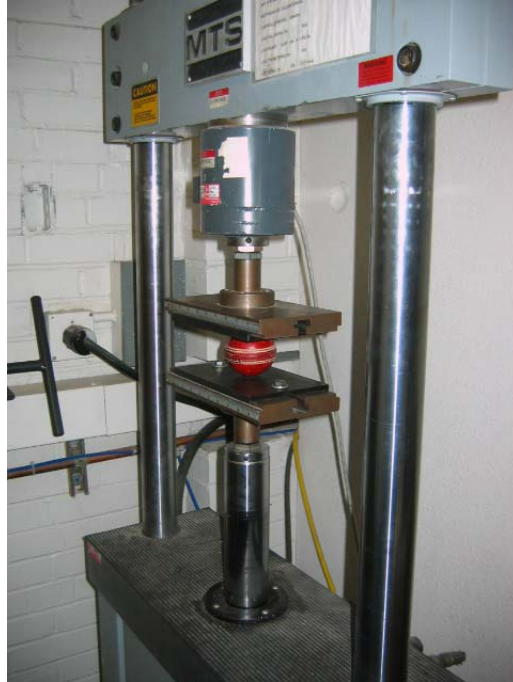
Figure 3.21: Face compression of the cricket ball.
