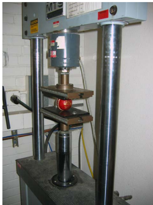
Figure 3.20: Seam Compression of the cricket ball.
