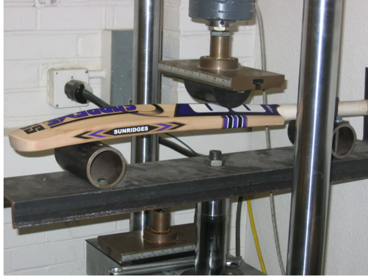
Figure 4.12: Cricket bat bending stiffness test.
