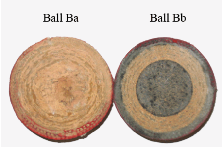
Figure 3.8: Cross sectional view of cricket ball Ba and Bb.
