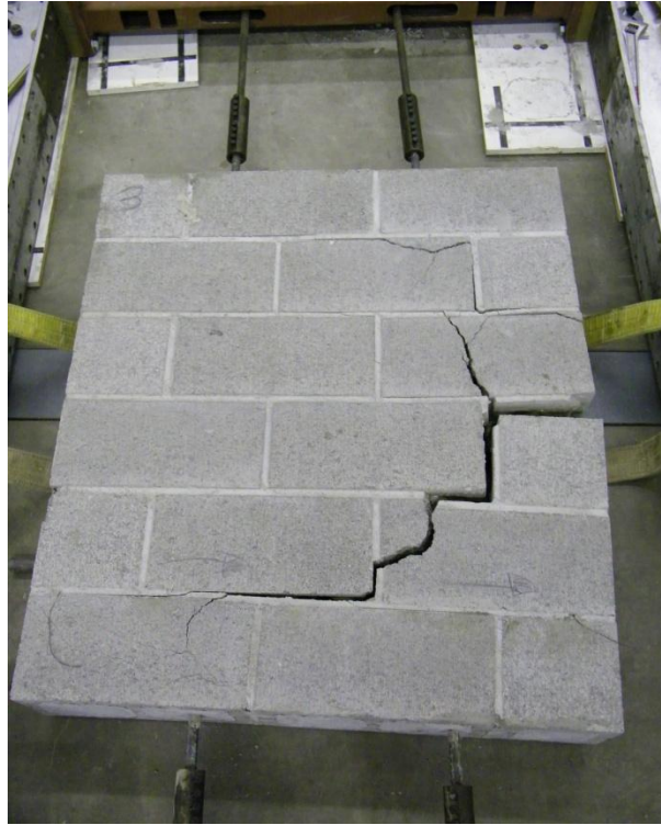
Figure 4.4. Typical Failure, Centered 36 db
