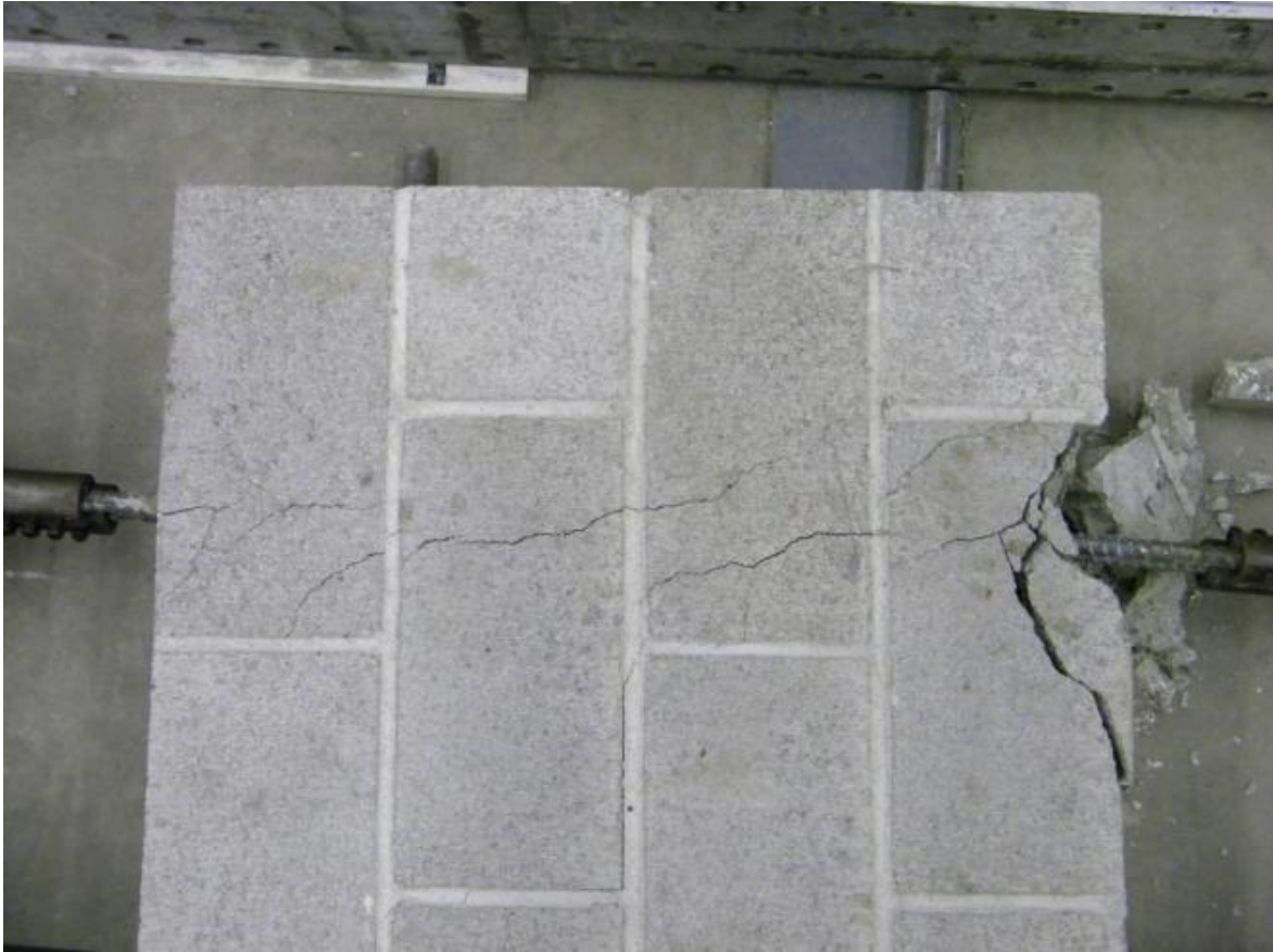
Figure 4.3. Longitudinal Cracking at Failure
