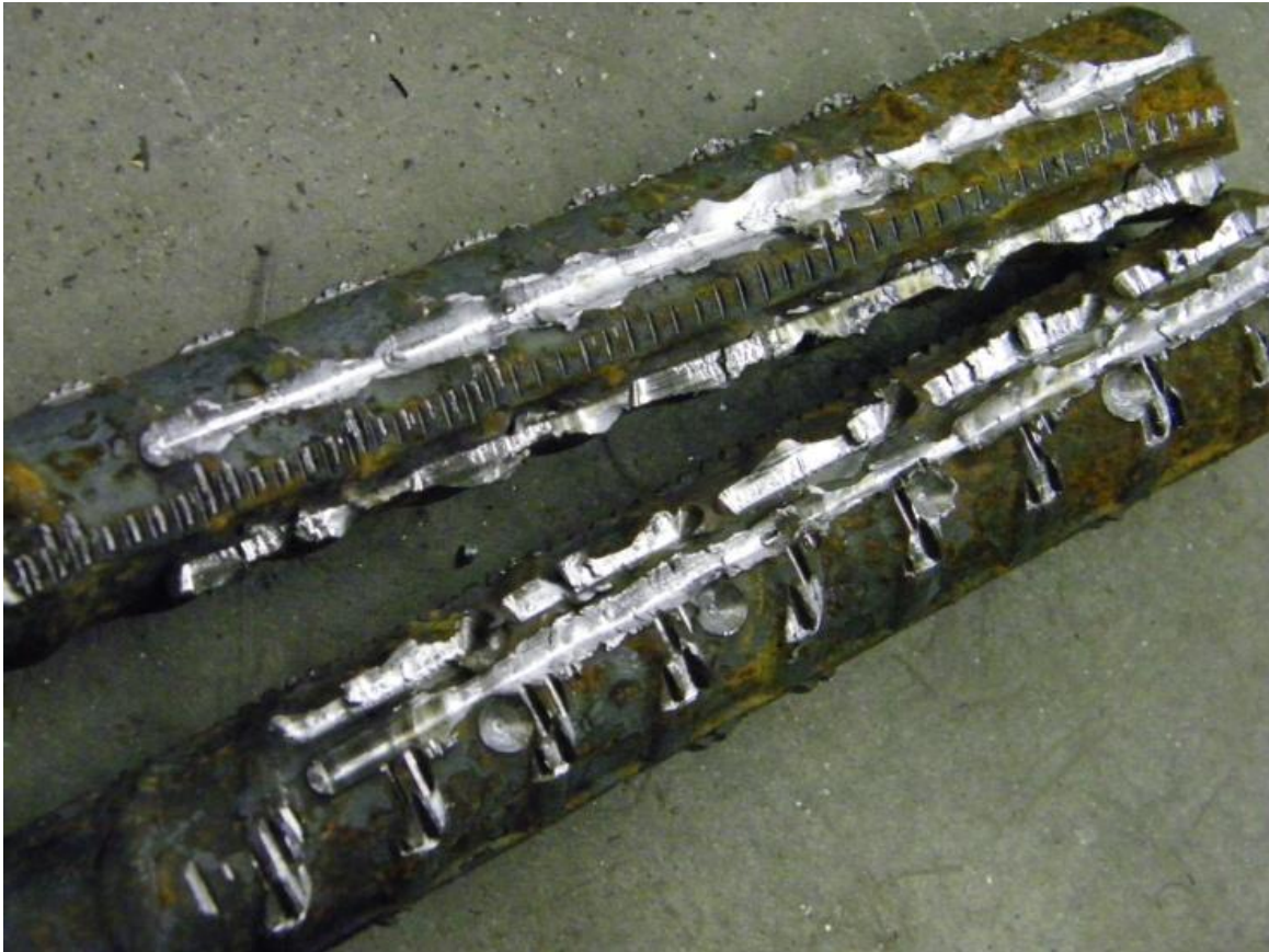
Figure 3.9. Damage in Coupler
