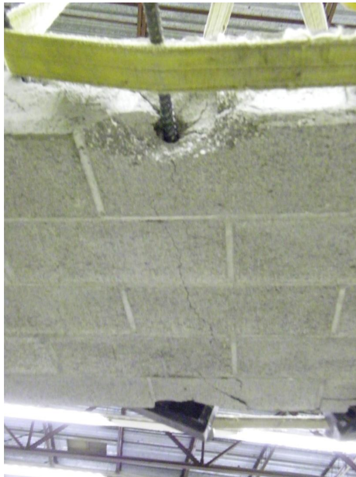
Figure 4.7. Typical Failure, Staggered Offset
