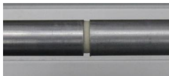
Figure 3.9 Installed Sample in Split Hopkinson Pressure Bar
