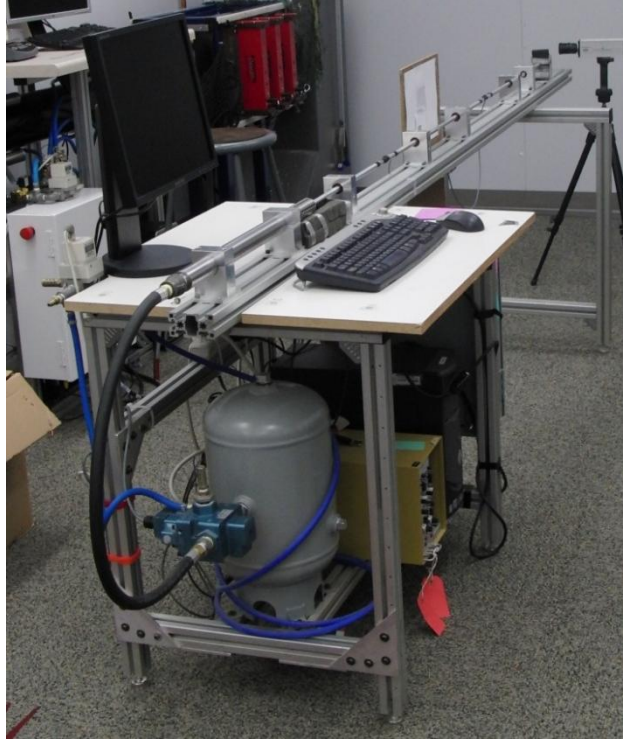
Figure 3.1 Split Hopkinson Pressure Bar Setup
