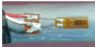
Figure 3.4 Mounted and Wired Strain Gage
