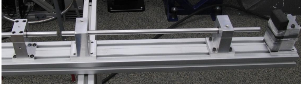
Figure 3.3 Momentum Trap on Split Hopkinson Pressure Bar
