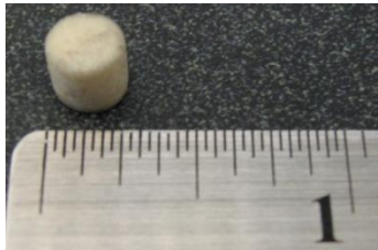
Figure 4.9 First Polyurethane SHPB Test Sample
