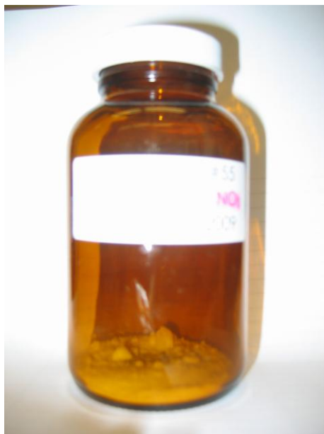
Figure 3: 250 mL amber glass jar containing 7g potassium nitrate crystals, prior to sediment addition.
