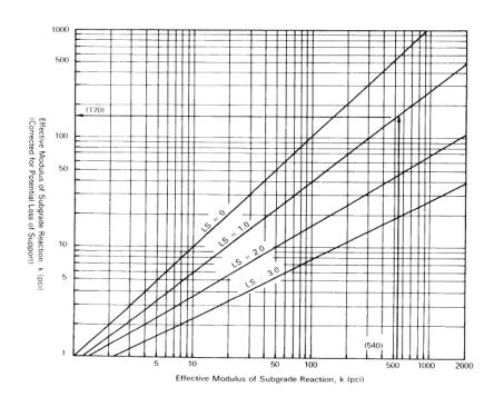
Figure 5.2: Correction of Effective Modulus of Subgrade Reaction for Potential Loss of Subbase Support (AASHTO, 1993 Figure 3.6)
