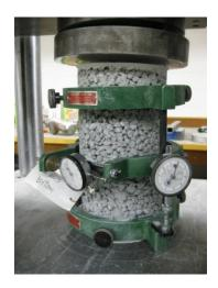
Figure 3.3: Modulus of Elasticity and Poisson's Ratio Test Set-up (9/16/09, Sloan Building, WSU)
