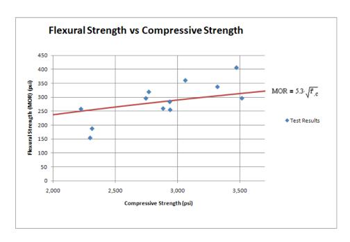
Figure 3.8: Relationship between Modulus of Rupture and Compressive Strength for Evolution Paving Beam Samples
