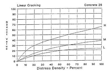
Figure 4.2: Linear Cracking Deduct Value Chart (ASTM D6433, 2007 Figure X4.8)
