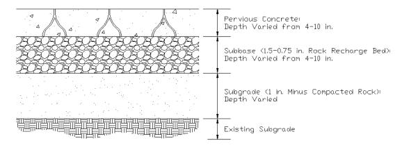
Figure 2.2: Typical Cross Section for Evolution Paving Pervious Concrete Panels
