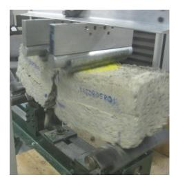
Figure 3.2: Failure of Beam Specimen during Third-Point Loading Test
