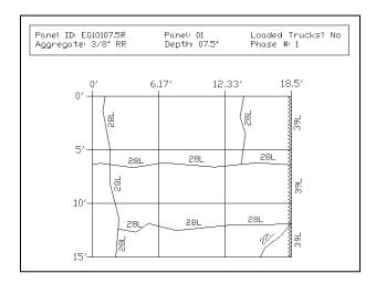
Figure 4.4: Example Distress Survey Results
