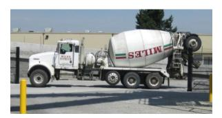
Figure 2.7: Fully Loaded Concrete Truck at Miles Sand & Gravel with Booster Axles Up
