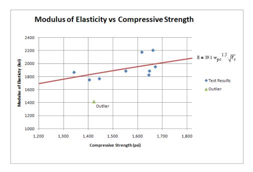
Figure 3.10: Comparison of Modulus of Elasticity and Compressive Strength for Laboratory Prepared (WE) Samples
