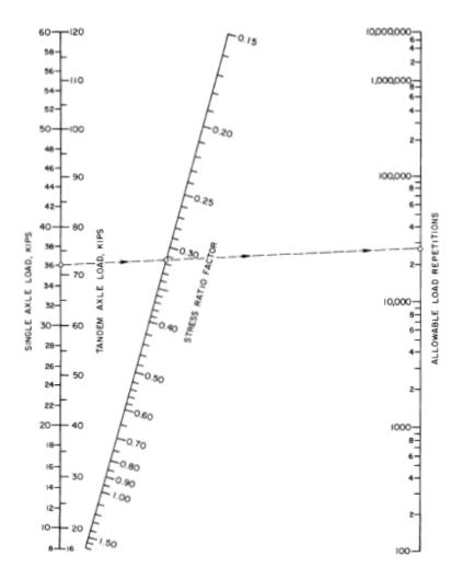
Figure 5.3: Fatigue Analysis - Allowable Load Repetitions Based on Stress Ratio Factor (PCA, 1984 Figure 5)
