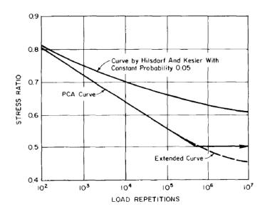
Figure 5.4: Fatigue Relationship for Concrete Used for the PCA (1984) Fatigue Analysis (PCA, 1984 Figure A.3)
