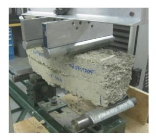
Figure 3.1: Third-Point Loading Test Set-up
