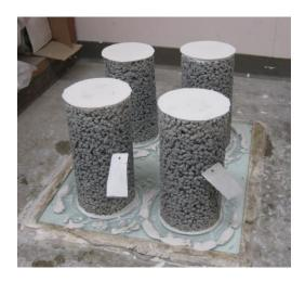
Figure 3.5: Gypsum Plaster Capping of Laboratory Prepared Pervious Concrete Samples (9/8/09, Sloan Building, WSU)
