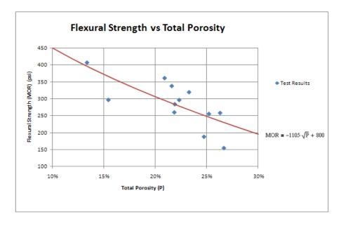
Figure 3.9: Flexural Strength versus Total Porosity for Evolution Paving Pervious Concrete Samples
