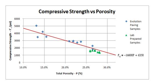
Figure 3.11: Relationship between Compressive Strength and Porosity
