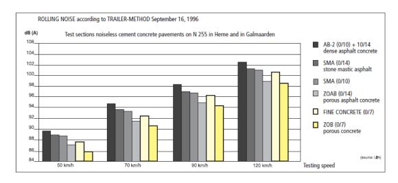
Figure 1.1: Road Noise of Different Pavements (Hendrickx, 1998)
