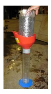
Figure 3.7: Exfiltration Rate Test Setup (7/7/09, Albrook Building, WSU)
