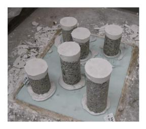
Figure 3.4: Gypsum Plaster Capping of Cored Pervious Concrete Samples (9/8/09, Sloan Building, WSU)
