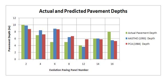
Figure 5.7: Comparison of Actual Pavement Depth at Evolution Paving with Pavement Depths Calculated with AASTHO (1993) and PCA (1984) design methods
