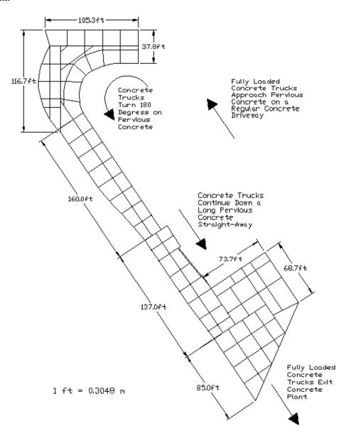
Figure 2.4: Pervious Concrete Driveway Layout at Miles Sand & Gravel in Kent, WA
