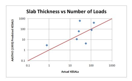
Figure 5.11: AASHTO (1993) Predicted ESALs versus Actual ESALs for Pervious Concrete at Evolution Paving (50% Reliability)
