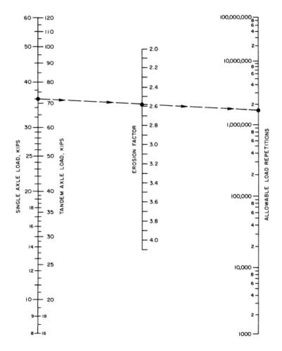
Figure 5.6: Erosion Analysis - Allowable Load Repetitions Based on Erosion Factor (Without Concrete Shoulder) (PCA, 1984 Figure 6a)
