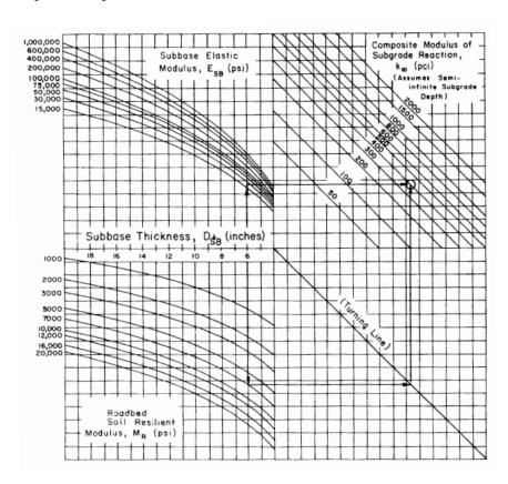
Figure 5.1: Chart for Estimating Composite Modulus of Subgrade Reaction (AASHTO, 1993 Figure 3.3)
