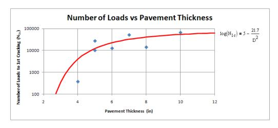
Figure 5.12: Number of Loads to 1st Cracking versus pavement thickness for Pervious Concrete Panels at Evolution Paving
