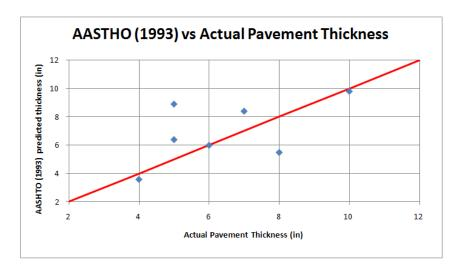
Figure 5.8: Predicted Pavement Thickness Based on AASHTO (1993) versus Actual Thickness for Pervious Concrete Panels at Evolution Paving
