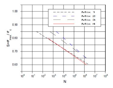
Figure 5.5: Fatigue Relationship Developed for Pervious Concrete (Pindado et al., 1999 Figure 4)
