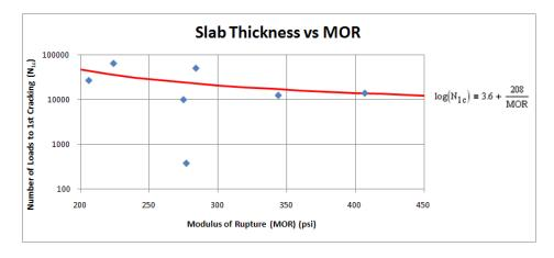
Figure 5.13: Number of Loads to 1st Cracking versus Modulus of Rupture for Pervious Concrete Panels at Evolution Paving
