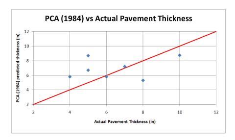
Figure 5.9: Predicted Pavement Thickness Based on PCA (1984) versus Actual Thickness for Pervious Concrete Panels at Evolution Paving
