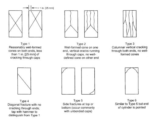
Figure 3.6: Typical Fracture Patterns for Compression Test (ASTM C 39, 2005 Figure 2)
