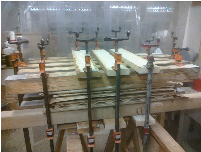
Figure 1.4.5: Clamping of wood-strand sandwich panels. Three panels were clamped at a time.
