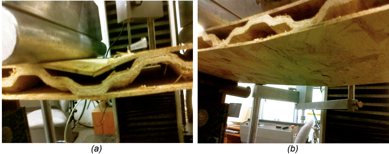
Figure 2.5.5: (a) Typical local ply failure for transverse specimens. (b) Flexural failure in transverse specimen.
