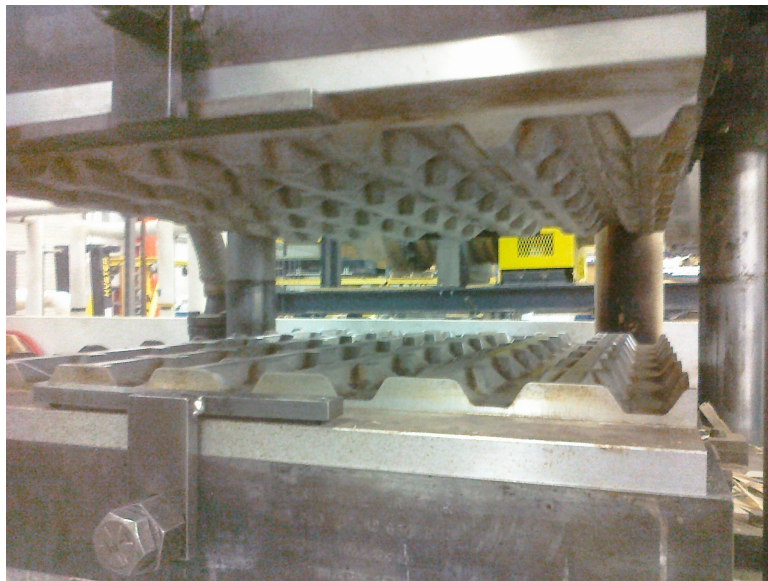
Figure 1.4.4: Hot press with 3-D mold installed.
