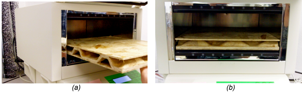
Figure 2.4.1: (a) Fox 304™ heat flow meter with 305 mm x 305 mm (12 in x 12 in) specimen. Note two of the three ribs being shown along the left wall of the chamber. (b) Chamber of Fox 304™ heat flow meter.
