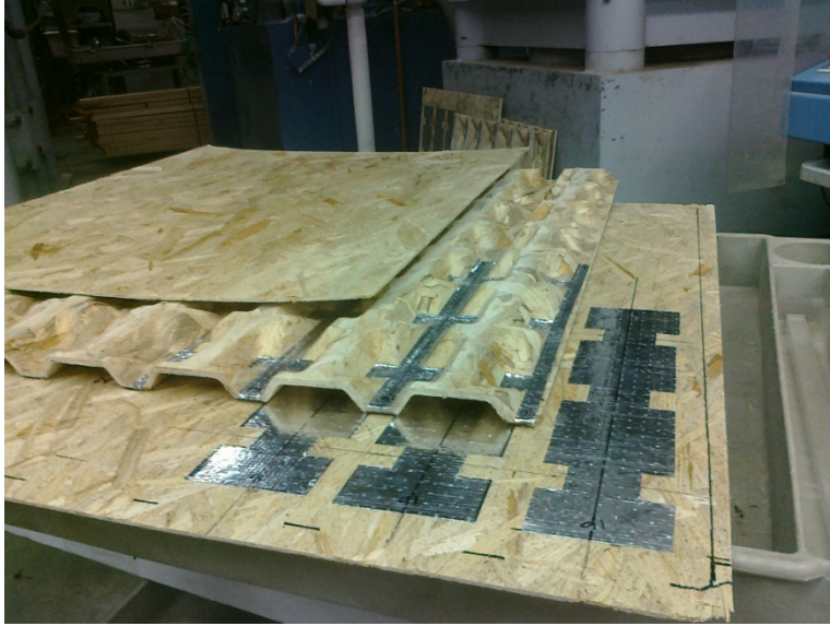
Figure 3.3.7: Typical installation of radiant barrier.
