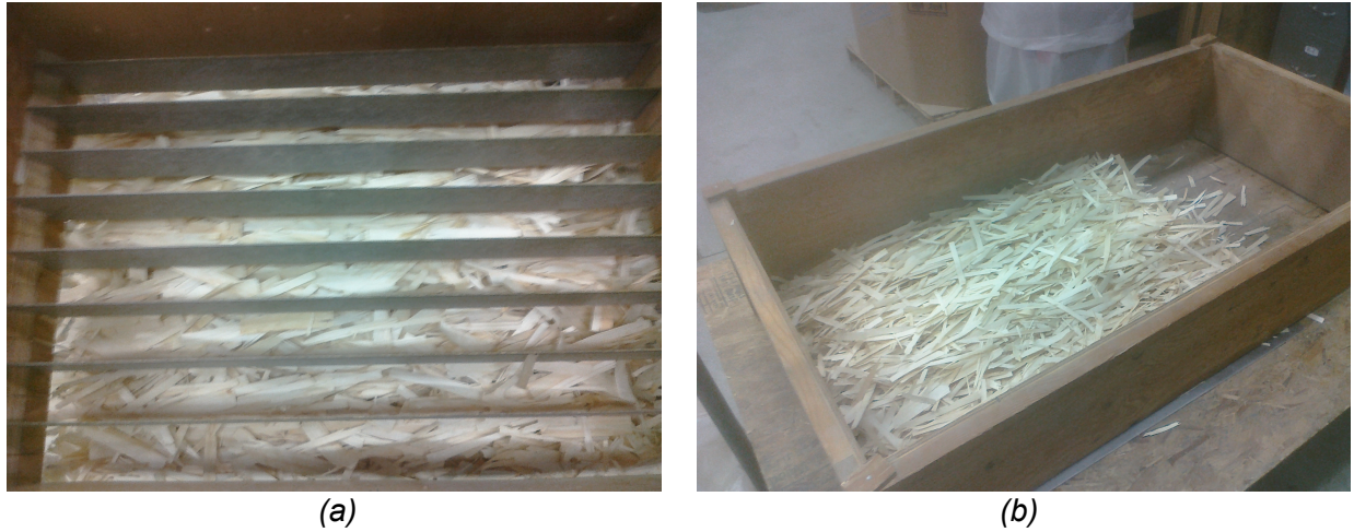
Figure 1.4.3: (a) Wood strand mat on shake table. (b) Form box utilized during mat formation.
