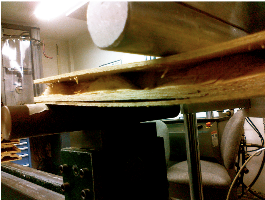
Figure 2.5.4: Failure of longitudinal specimen. Note typical delamination failure as well as the occasional flexure failure in the core located below the load bar.
