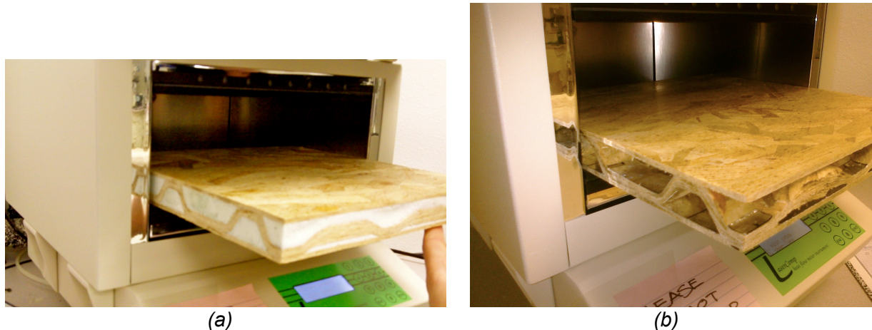
Figure 3.3.8: (a) Foam incorporated wood-strand sandwich panel. (b) Radiant barrier incorporated sandwich panel. Note the radiant barrier on bottom near the hot plate.
