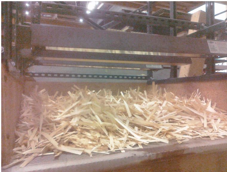
Figure 1.4.1: Wood strands drying in box dryer.
