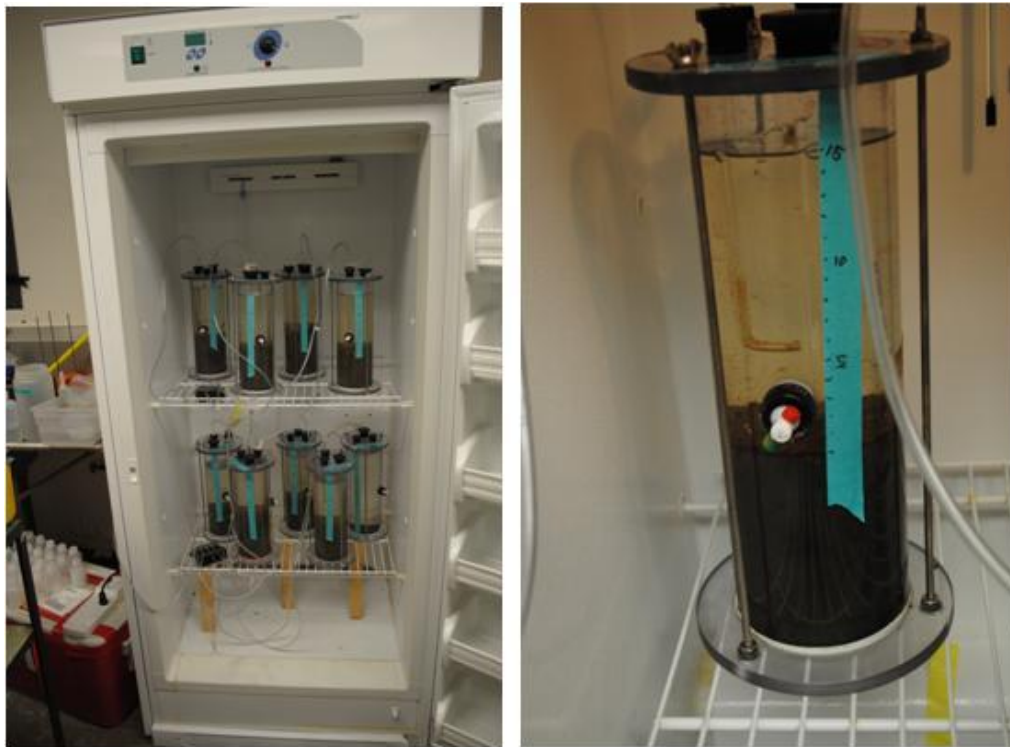
Figure 2.3: Sediment-water interface chambers in incubation with bubbling air mixture.
