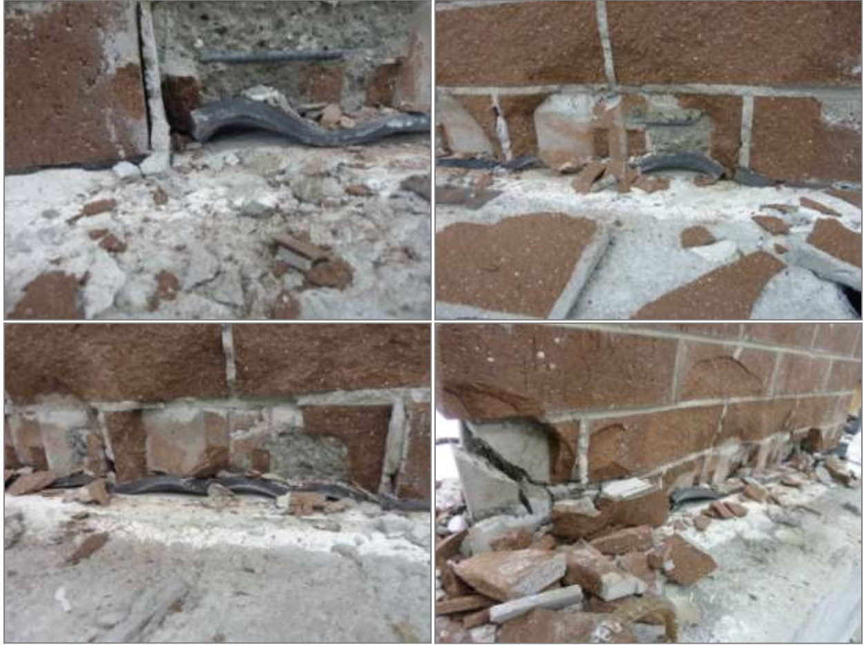
Figure 5.6: Neoprene Friction Reaction in Panel 2
