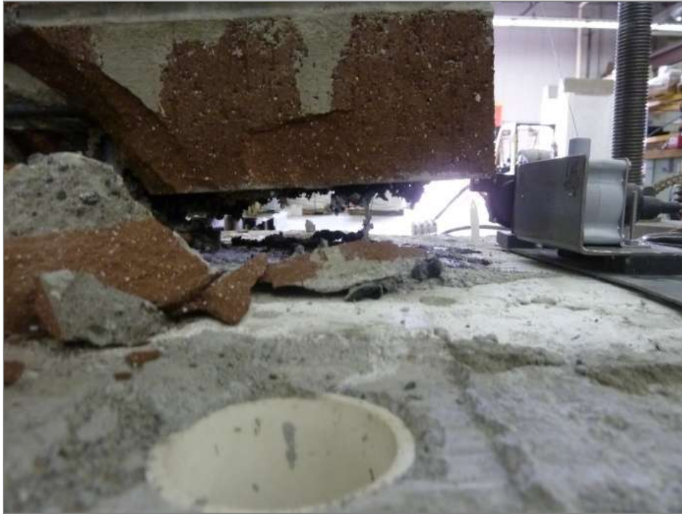
Figure 4.13: Uplift at North Toe
