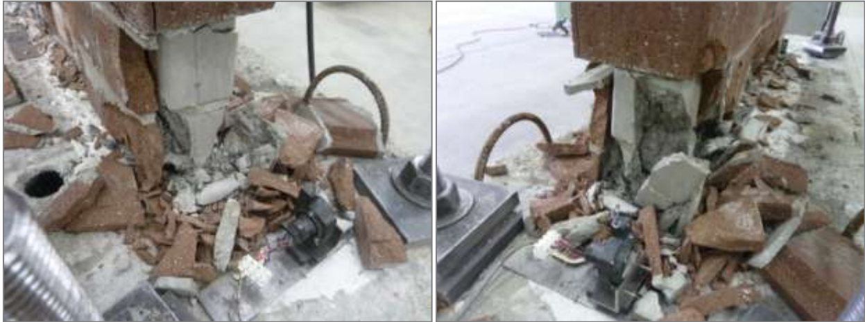
Figure 4.15: Toe Crushing at South Toe
