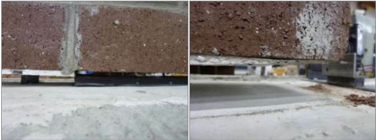
Figure 4.3: Uplift of the North and South Ends of the Panel
