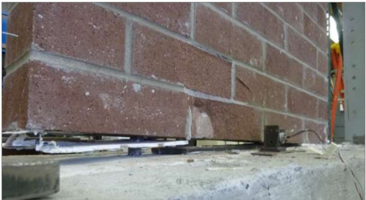
Figure 4.2: Rocking Behavior and Uplift of One End
