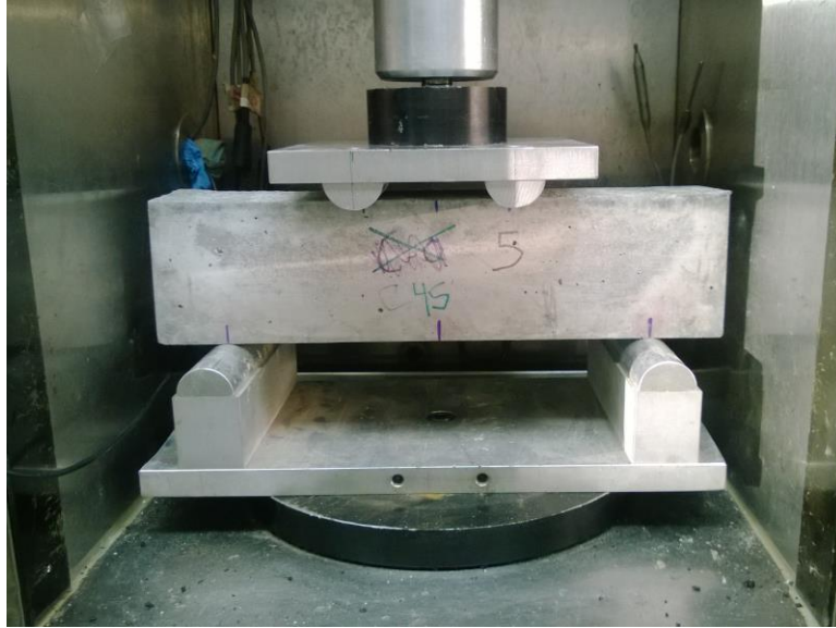
Figure 3.1 Nonstandard Flexural Modulus with Third Point Loading Test Setup
