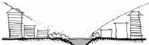
Fig. 28 Building Height Reduced closest to Spokane River (9).
