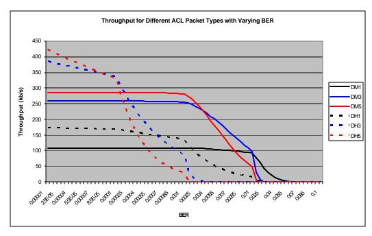
Figure 3.1: Bluetooth ACL Packet Throughput, Symmetric Channel
