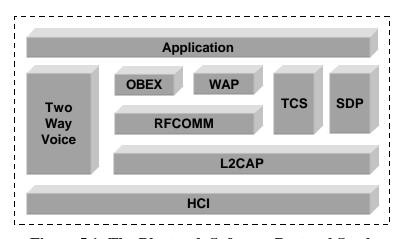
Figure 5.1: The Bluetooth Software Protocol Stack
