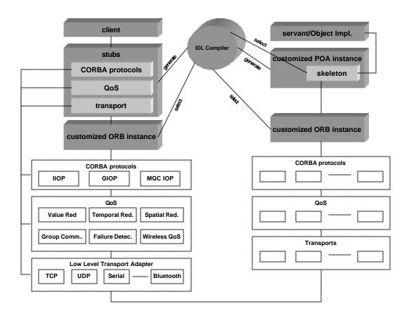
Figure 2.1: MicroQoSCORBA Architecture
