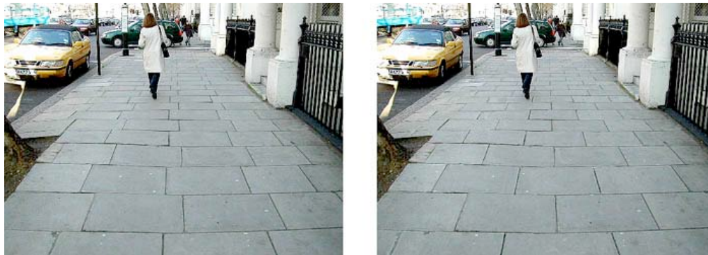
Figure 2-4. At left, offset joints in the paving stones of a London sidewalk subtly reinforce the direction of travel; at right, a retouched photo for comparison. (author, retouched by author)
