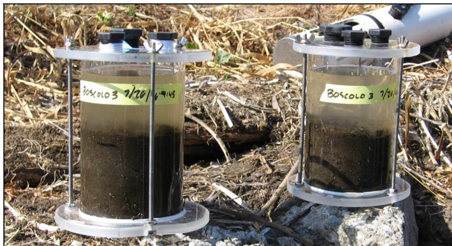
Figure 3-7 Freshly sampled sediment cores with their caps in place
