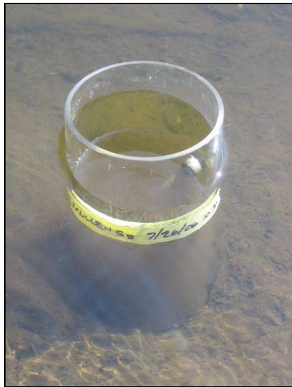
Figure 3-6 Sediment sampling chamber inserted into sediment-water interface prior to capping
