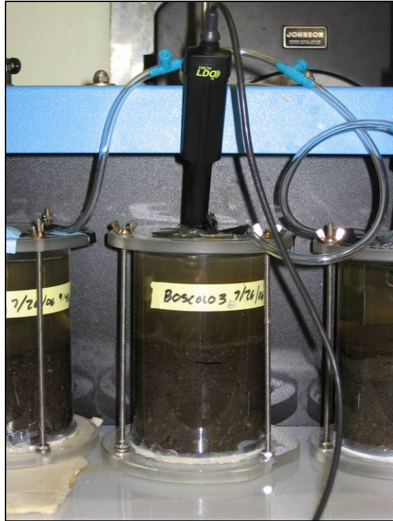
Figure 3-8 Lab set-up with probes, paddles, and aerating tubes installed
