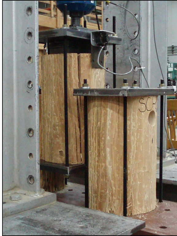
Figure 2.3 Cyclic connection test setup illustrating steel plate fixtures used as hold downs on the outer logs and load application for the middle log.
