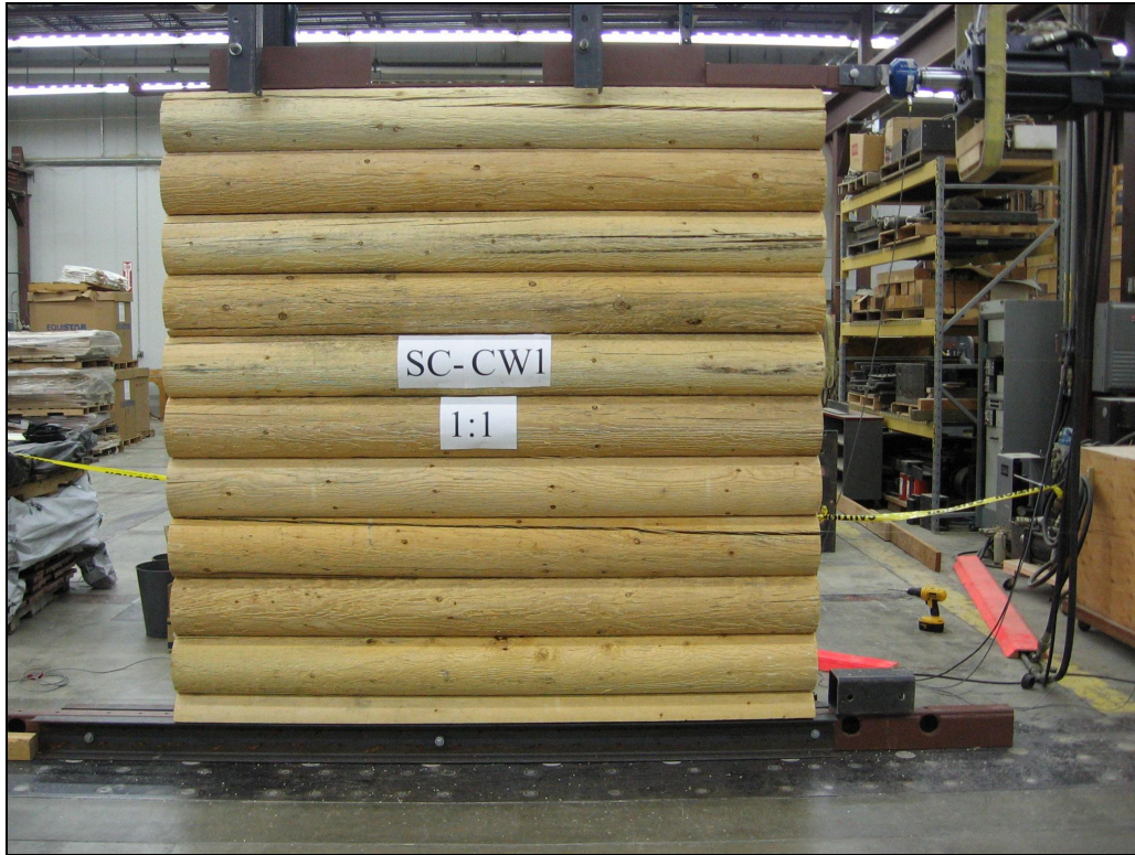
Figure 3.3 Overall test setup (Note: Wall shown has 1:1 aspect ratio).
