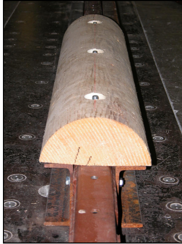
Figure 3.1 Sill log attachment to rigid floor beam.
