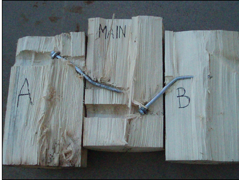
Figure 2.5 Cross-section of connection utilizing 254x12.7 mm lag screws following a monotonic connection test.
