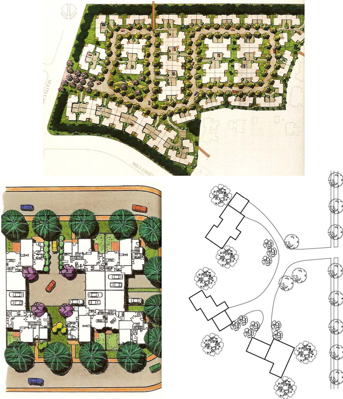
Figure 2.2-11. Shared parking configurations. The narrow roadway connecting driveways in the lower right diagram is considered part of the driveway system and typically does not have to meet standard road design criteria. (Sources: Top and bottom left - Fader, 2000, pp. 30 & 32. Bottom right - Author, adapted from CWP, 1998, p. 116)
