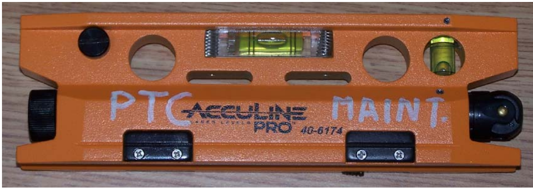
Figure 9.1: Laser Level for Position Measurements
