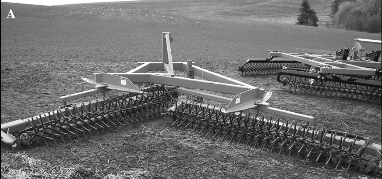
Figure 1.5. The rotary harrow, typically a secondary tillage tool used for residue management, has potential use as a primary tillage tool in mulch-tillage conservation tillage. The Phoenix ® model has two adjustable axles (a), each made of interwoven, blunt-ended metal rods (b). (Photos taken by S. Kopan)
