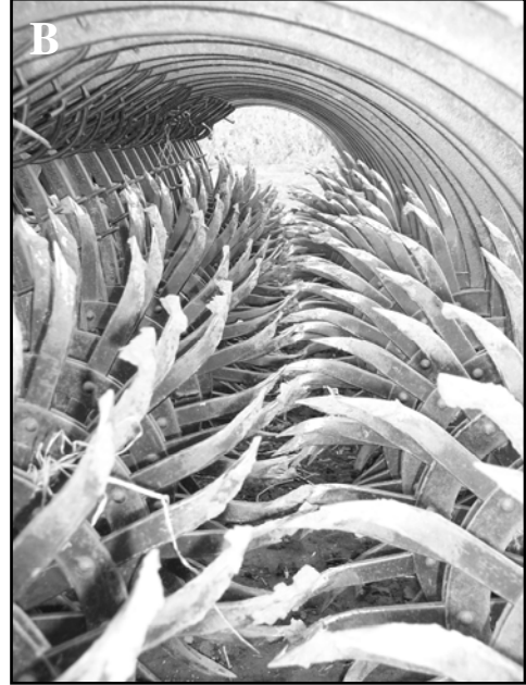
Figure 1.6. The rotary hoe is used for secondary tillage operations. The M&W© Minimum Tillage rotary hoe has two rows of spinning wheels, offset to prevent residue clogging (a). Each wheel has a spooned ends, which uproots emerging weeds within 5 cm of the soil surface (b). (Photos taken by S. Kopan)
