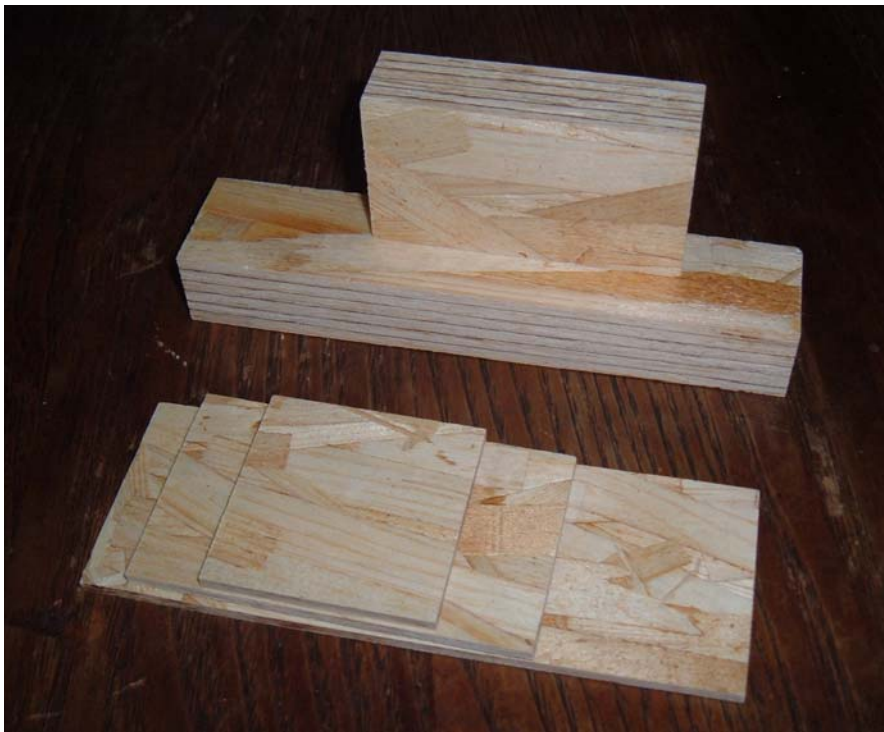
Figure 2.1. Thin strand plies and laminated strand ply (LSP) composites
