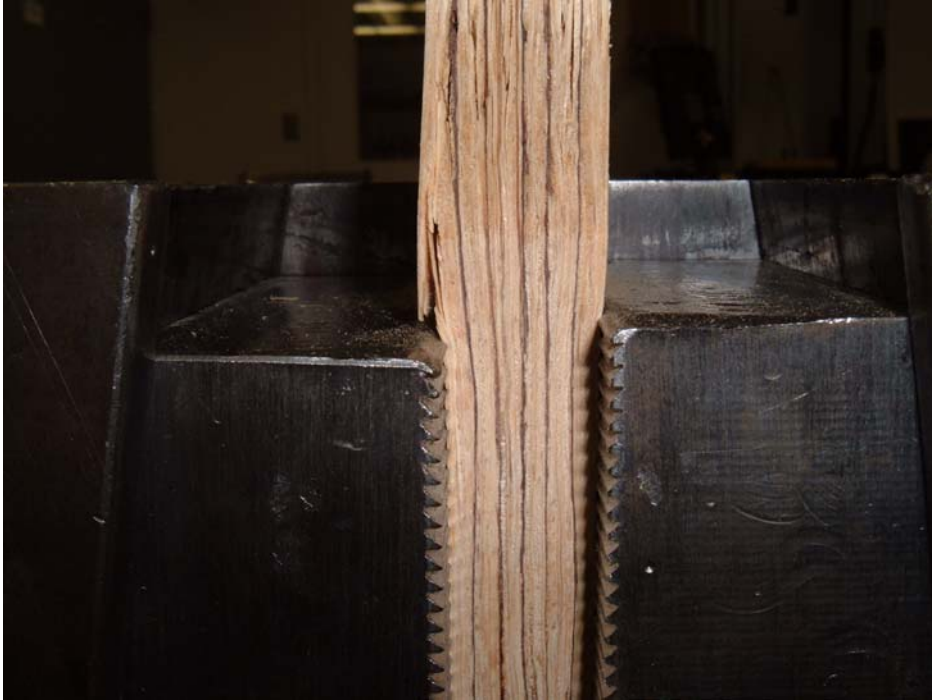
Figure 3.8. Failure of tension specimen initiating at the grips
