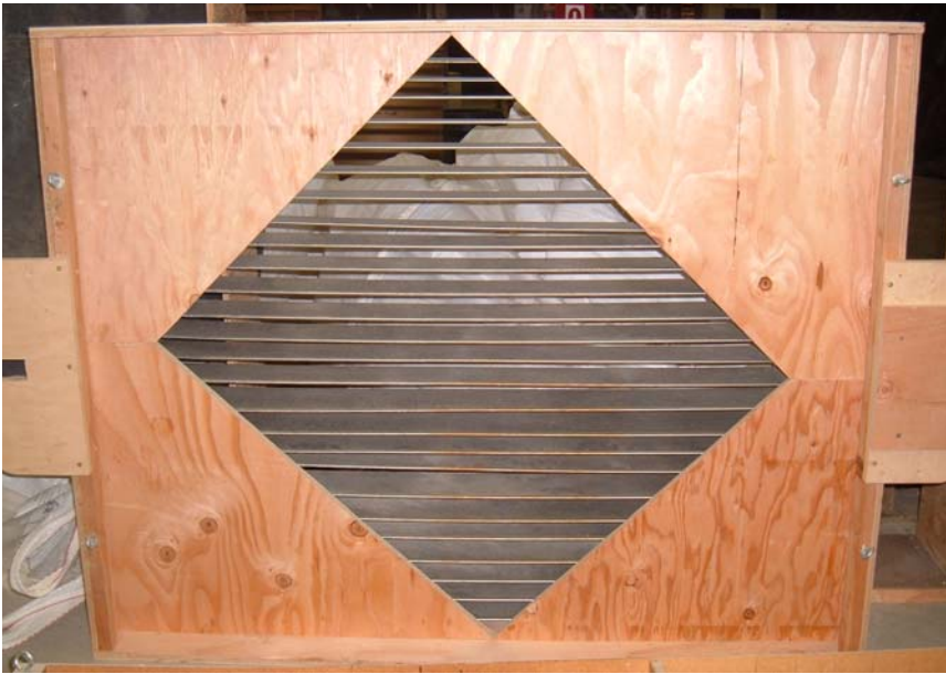
Figure 3.5. Forming box for 45 degree strand plies
