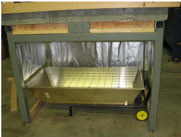
Figure 3.6 – Test set-up showing infrared heater and test frame supporting a concrete specimen
