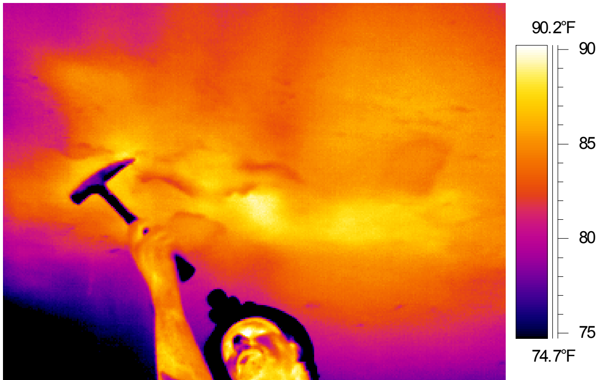
Figure 4.22 – Thermal image of Heating Location # 1: excavating a detected flaw
