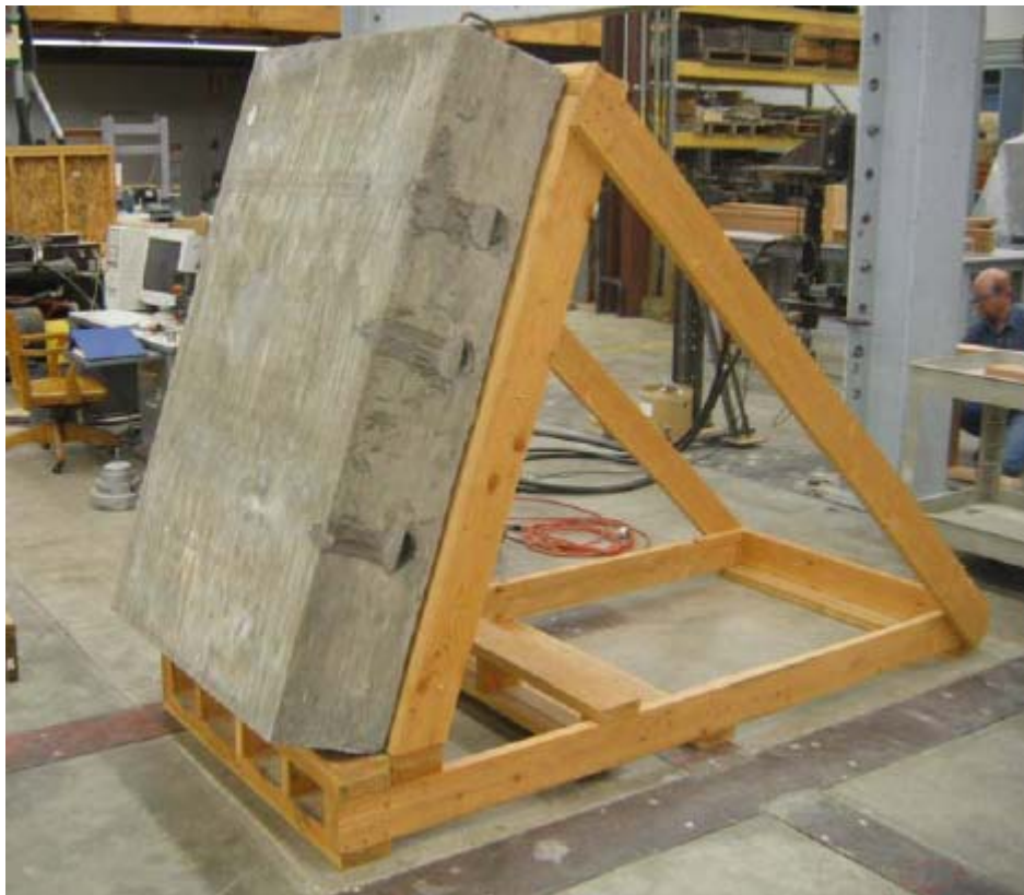
Figure 2.2 – Wooden test frame with concrete specimen (Musgrove 2006)
