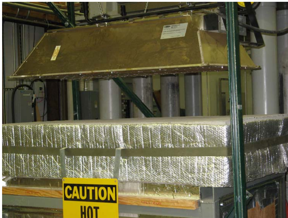
Figure 3.8 – Test set-up with heater suspended above a concrete specimen
