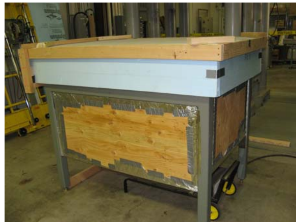
Figure 3.7 – Test set-up showing aluminum-covered plywood sides and insulation on edges/ends of a concrete specimen
