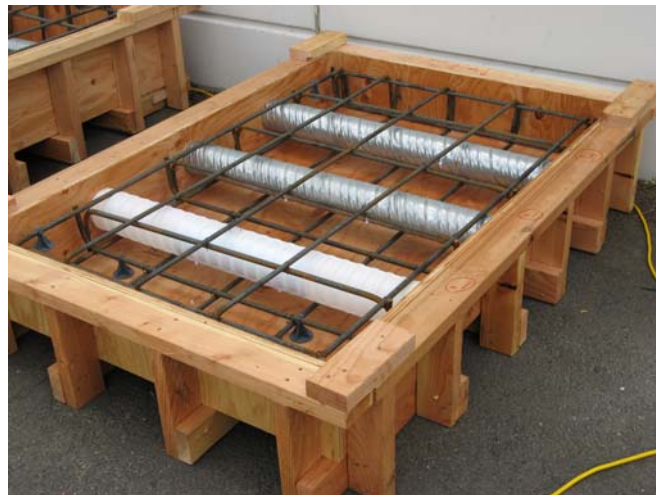
Figure 3.3 – Typical specimen formwork with post-tensioning ducts and rebar cage
