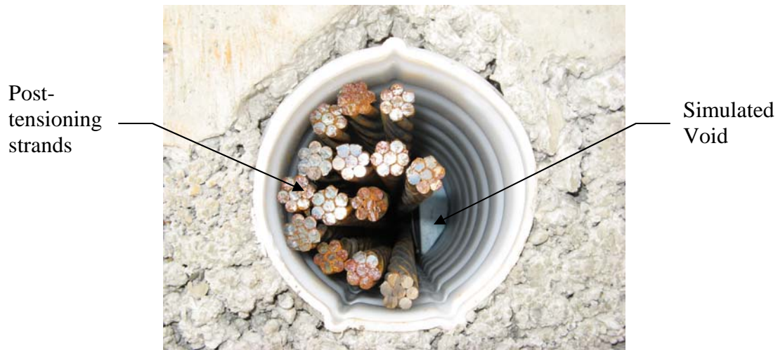
Figure 3.2 – Typical 7-wire strands and simulated void in post-tensioning duct
