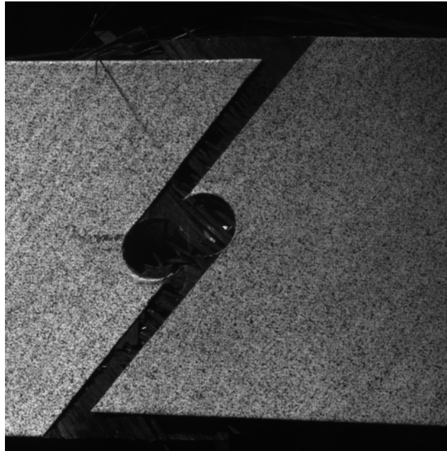
Figure I.1: Layup A at Failure
