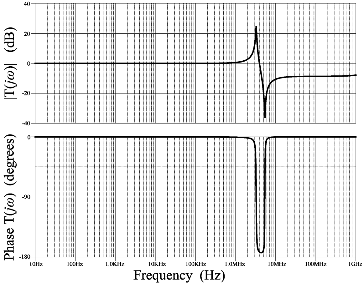
Figure 5-41: Drive to sense winding transfer function Bode plots for the typical parasitics of isolation transformer circuit.
