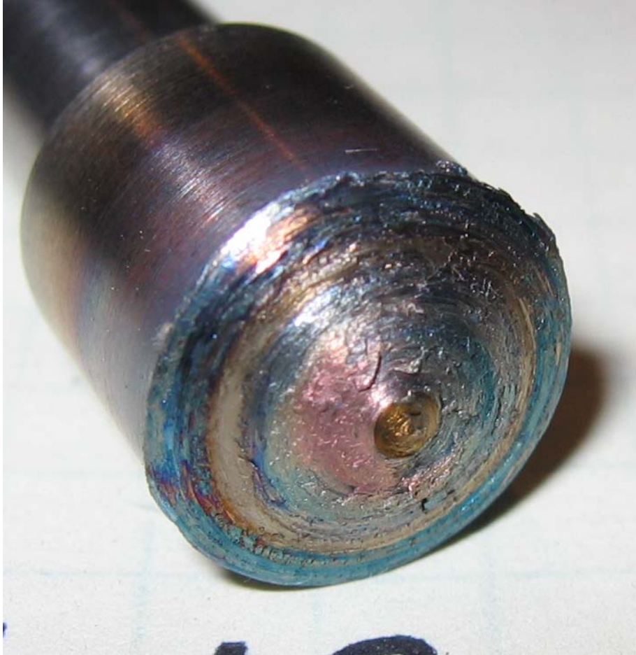
Figure 11. H-13 friction stir welding tool after three plunges in titanium sheet alloyed with 20% atomic hydrogen.
