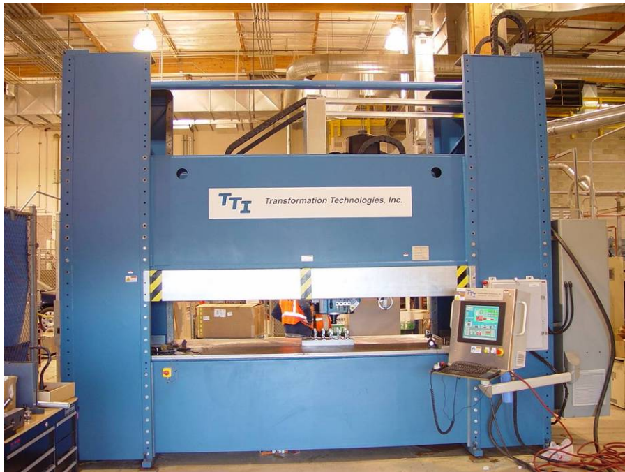
Figure 4. High stiffness friction stir welding machine located at the Pacific Northwest National Laboratory in Richland Washington.
