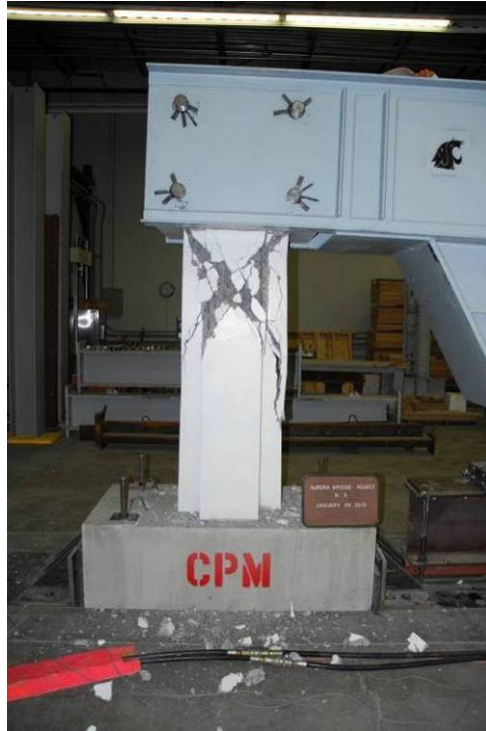
Figure 5.3.3 – Column 5 Shear Cracking Near the End of Testing.
