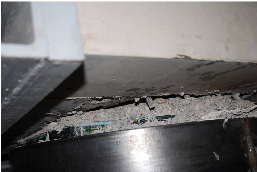
5.6.3 – Column 4 Longitudinal Rebar Fracture
