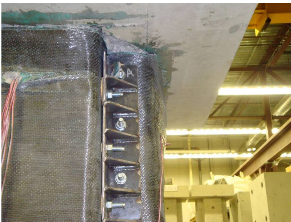
Figure 5.5.3 – Column 3 Bulging of FRP Jacket at the Top of the Column
