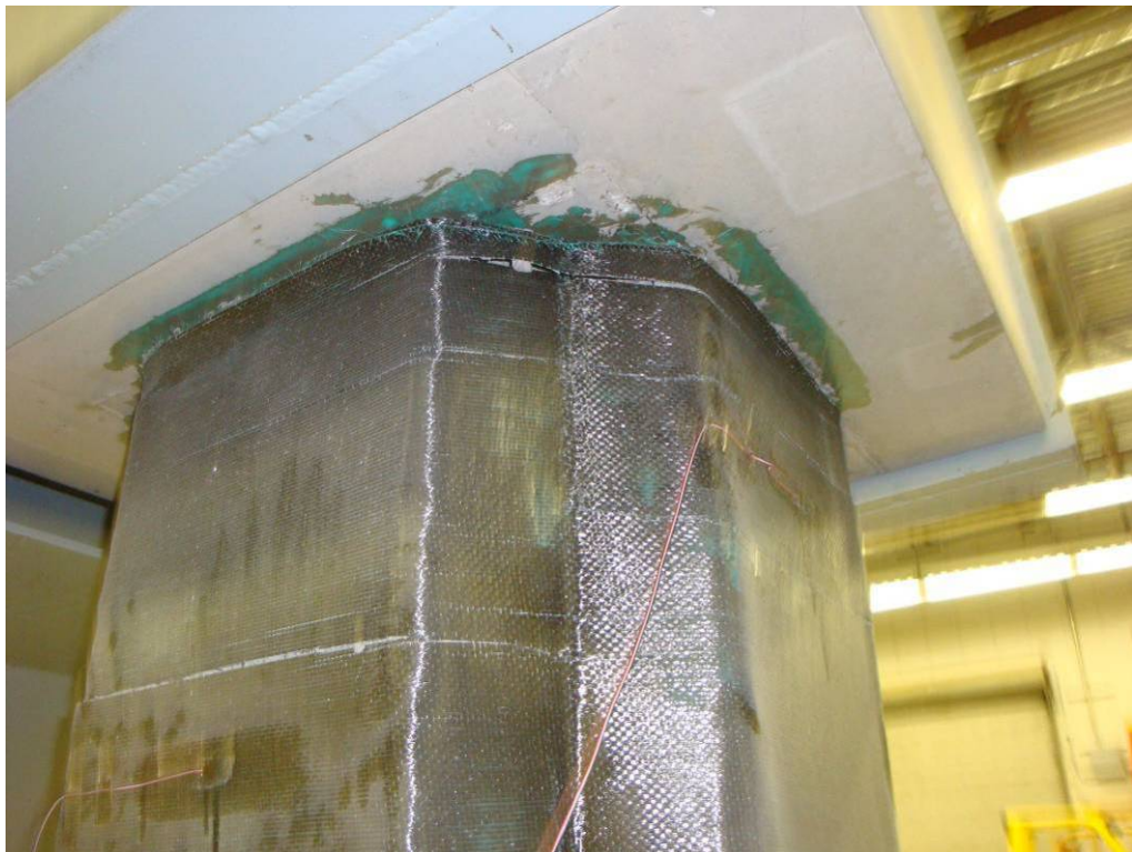
Figure 5.4.3 – Column 2 Pullout of FRP Jacket from Reentrant Corners
