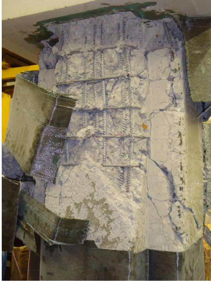
Figure 5.4.4 – Column 2 Large Shear Cracks under FRP Jacket at the End of Testing
