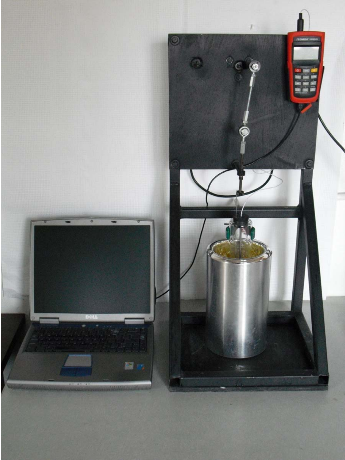
Photograph of freezing point apparatus built in accordance with ASTM D 1177.
